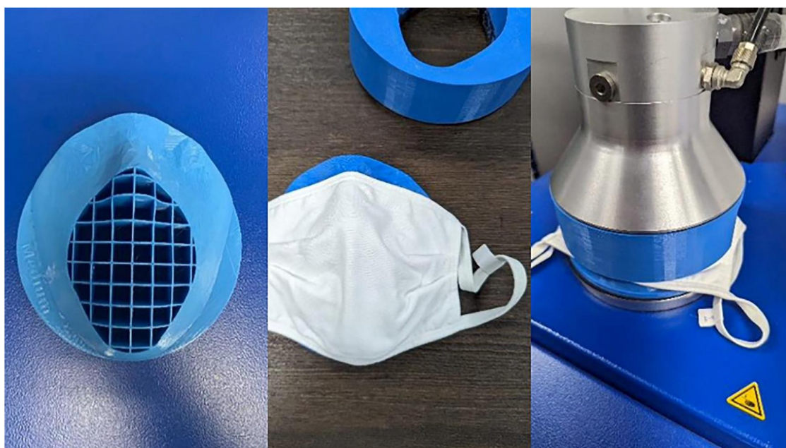
Figure 3. ASTM F3502-21 testing with the printed adult medium face form, mounted sample, and test setup from Intertek.
