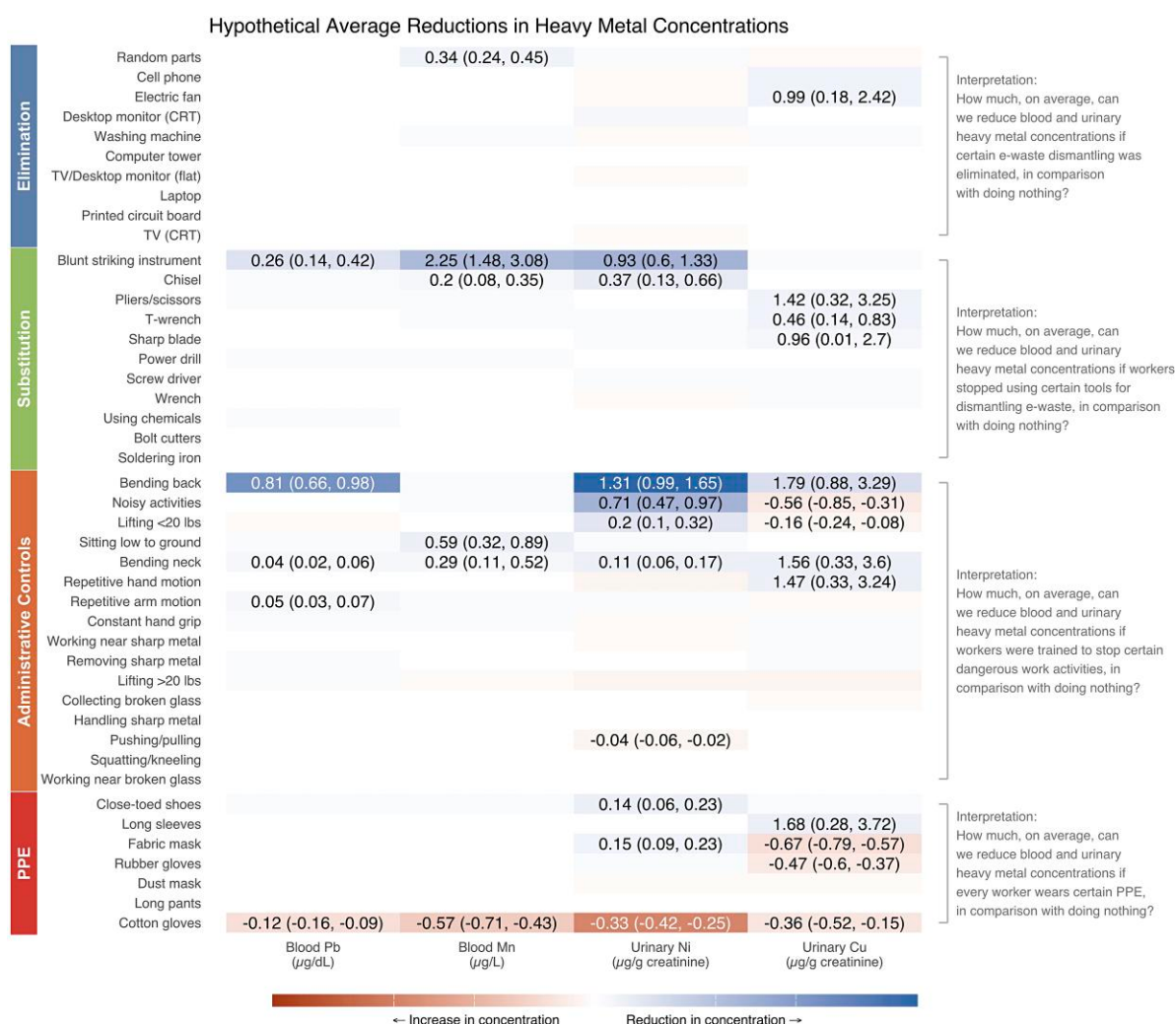
Fig. 3. Estimated average reductions in 4 heavy metal concentrations from hypothetical workplace controls. Hypothetical reductions were estimated from 4 random forest models (1 for each heavy metal) using the 44 workplace controls as predictors after accounting for selection bias using inverse probability weighting. Only reductions/increases that were statistically significant and had > 1% difference are presented in the figure.
