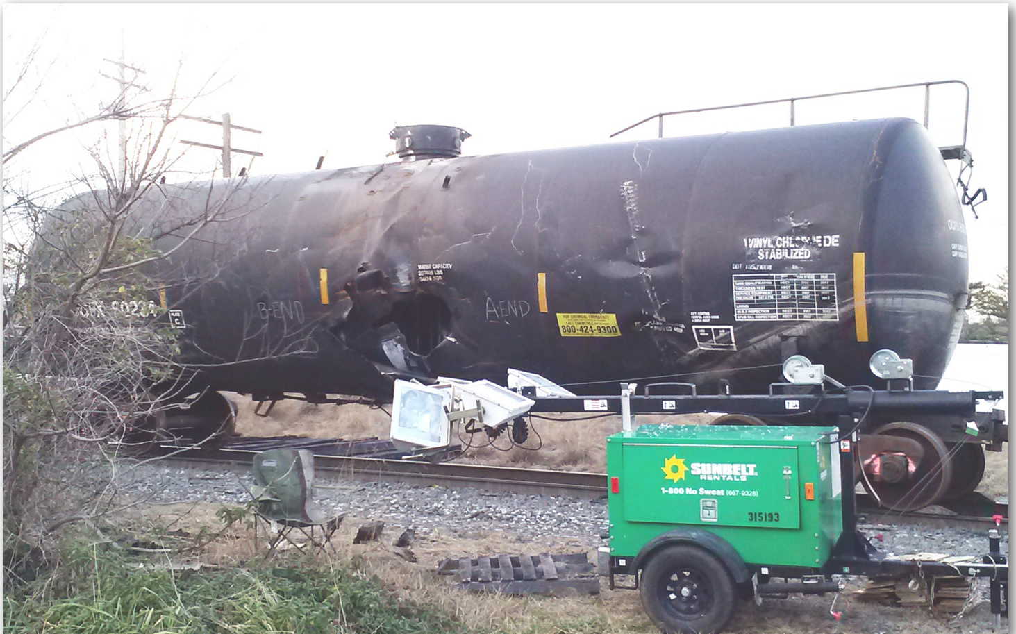
Hole in tanker car from vinyl chloride incident in New Jersey. Photo by: Mary Anne Duncan.
