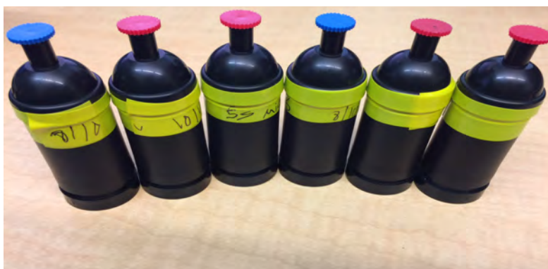
Figure 14: Filter Breathing Zone Samples
