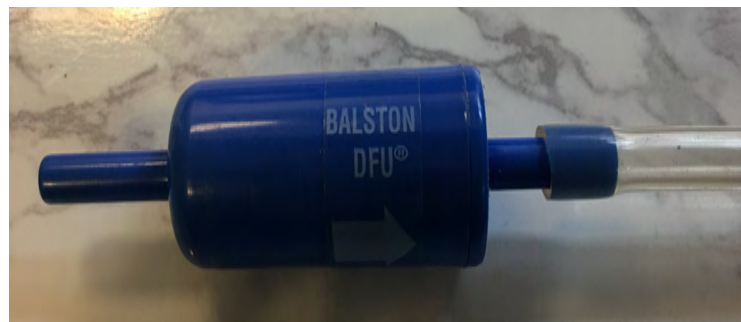
Figure 10: Zero Filter for CPCs
