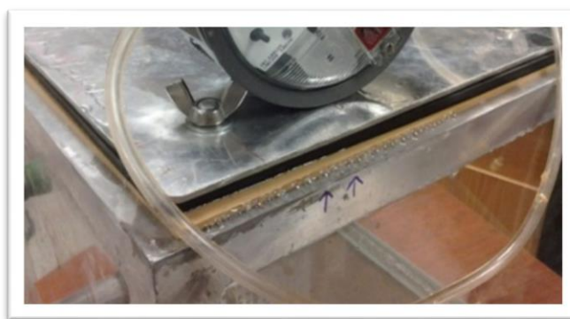
Figure 3. Air bubbles from leak in test chamber door.
