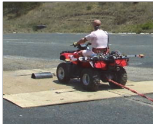
Figure 4. Bump obstacle perturbation test (Grzebieta et al., 2015b).
