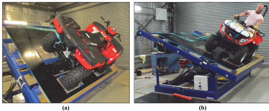
Figure 2. (a) Static ATV stability tests with a single-axis tilt table and (b) typical ATV setup with test dummy, front load, and rear load (Grzebieta et al., 2015c).
