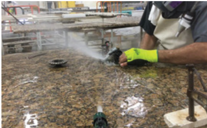
Figure 3. Sheet water wetting is an effective engineering control for RCS exposure during stone countertop grinding. From NIOSH: bit.ly/niosh-comp-report (PDF).
