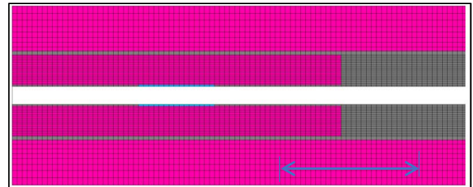
(B) After gauge installation (blue arrow) and overcoring. Grey=excavated elements. Gauge length blue) is 3.6d . Distances before and after gauge ends are 6d . The mesh is 823 mm (32.4 inches) long. Length of overcoring a gauge is 594 mm (23.4 inches)
