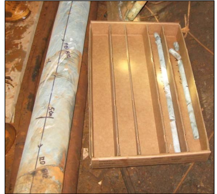
Figure 6. Photograph of large overcore of amphibolite at the Homestake site on the 4850 Level.
