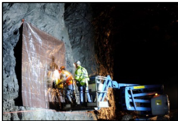
Fig. 5 3D GPR survey conducted along the Pillar-X
