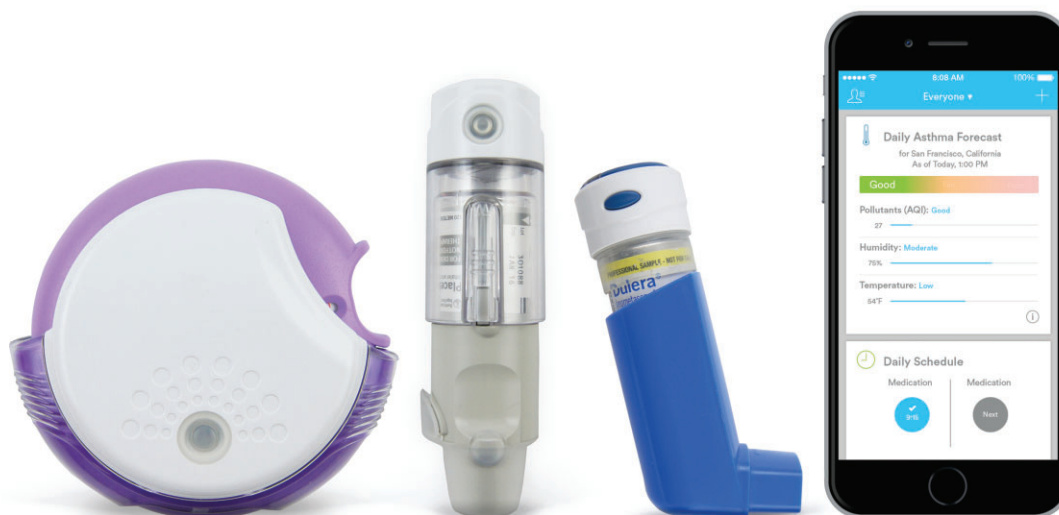
Figure 2 Digital medication sensors fit onto inhaled respiratory medications and record the date and time of use. Data are transmitted wirelessly via a paired smartphone
