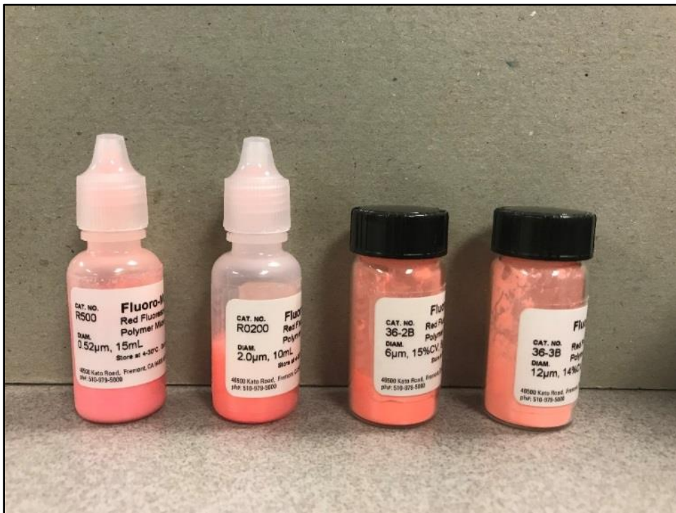
Figure 1: 0.5 \mu\text{m} and 2.0 \mu\text{m} FPLS Liquid Suspensions (Pictured Left) 6.0 \mu\text{m} and 12.0 \mu\text{m} FPLS Dry Powders (Picture Right).
