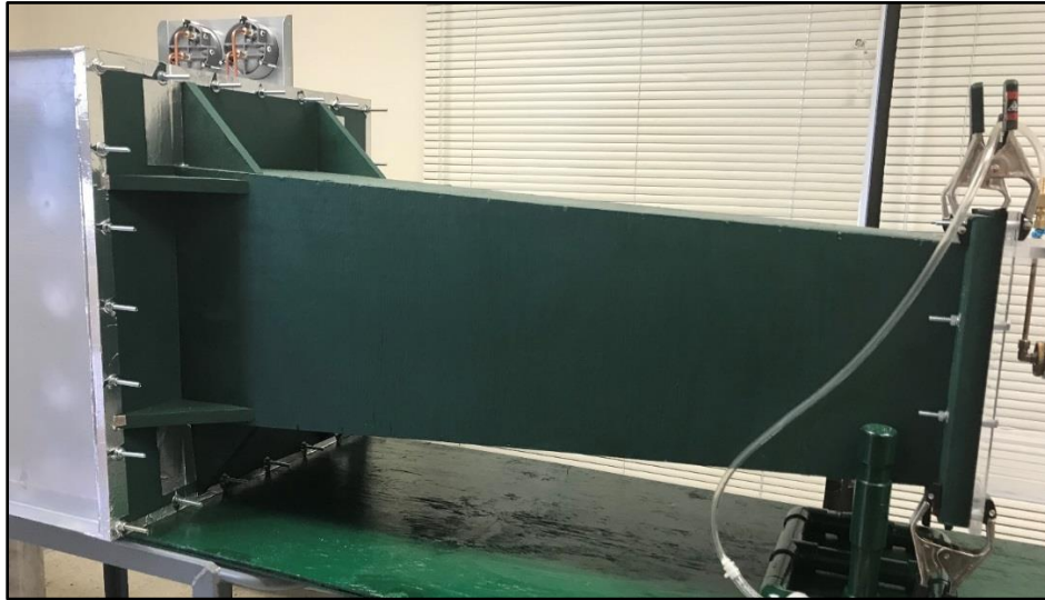
Figure 19: Wind Tunnel Diffuser.
