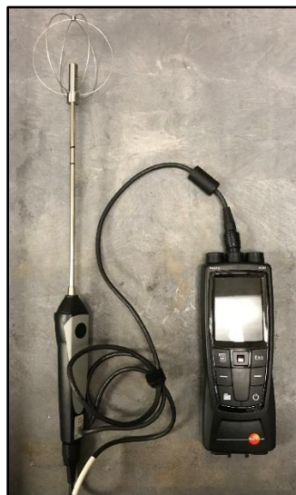
Figure 24: Testo Model 480 High End IAQ Measuring Instrument and the Degree of-Turbulence Probe.
