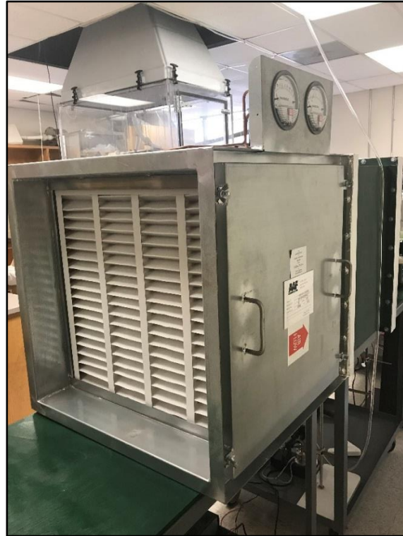
Figure 10: Wind Tunnel Entrance Filter Housing.
