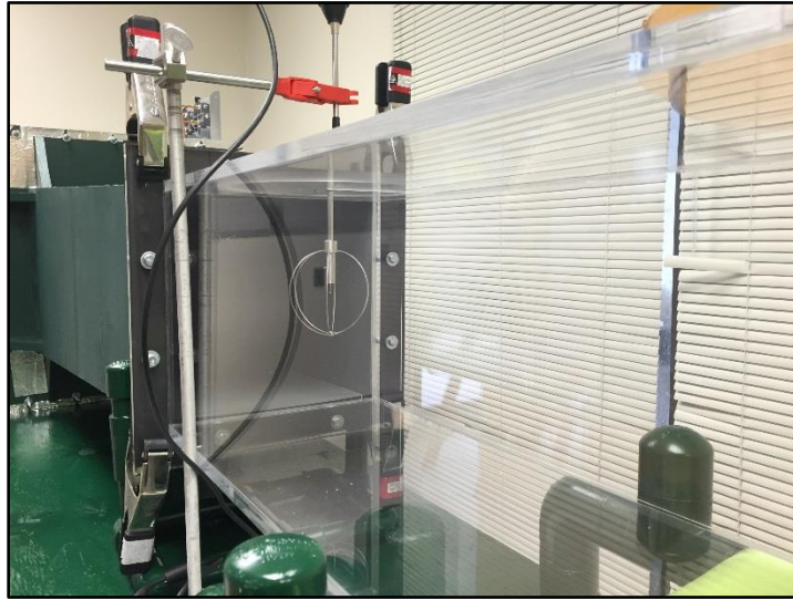
Figure 25: Testo Model 480 High End IAQ Measuring Instrument and the Degree of Turbulence Probe inside the Wind Tunnel.
