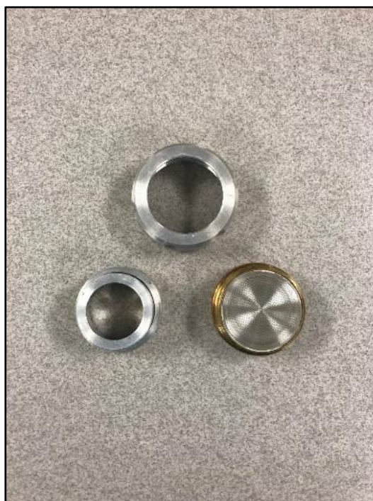
Figure 28: 1 Inch Isokinetic Sampling Probe Disassembled.
