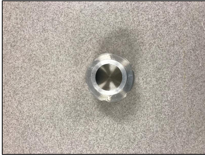
Figure 29: 1 Inch Isokinetic Sampling Probe Assembled.
