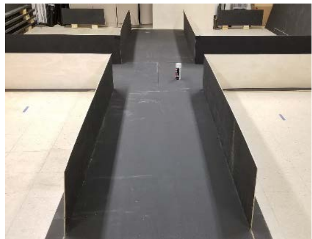
Figure 1. Simulated mine floor and ribs.
