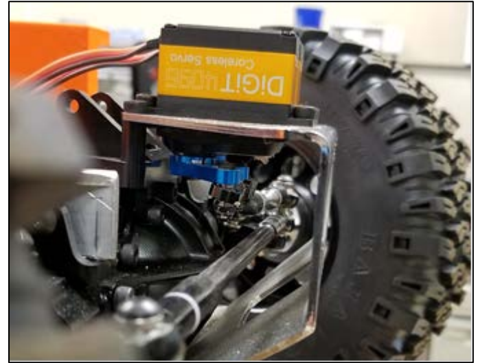
Figure 11. 1/6 th scale shuttle car steering servomotors.
