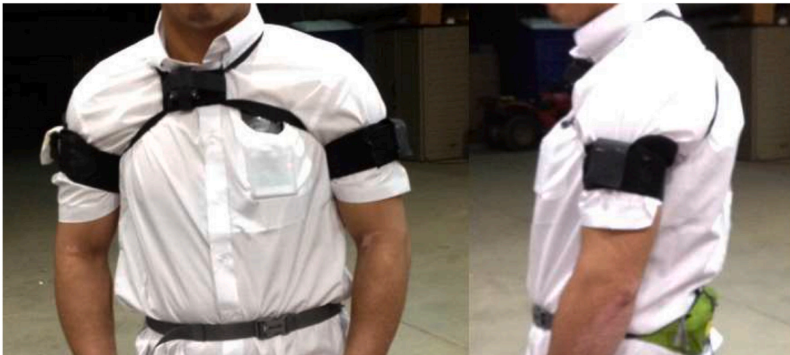
Fig. 4. Accelerometers attached to Participant's Upper Arms and Torso.
