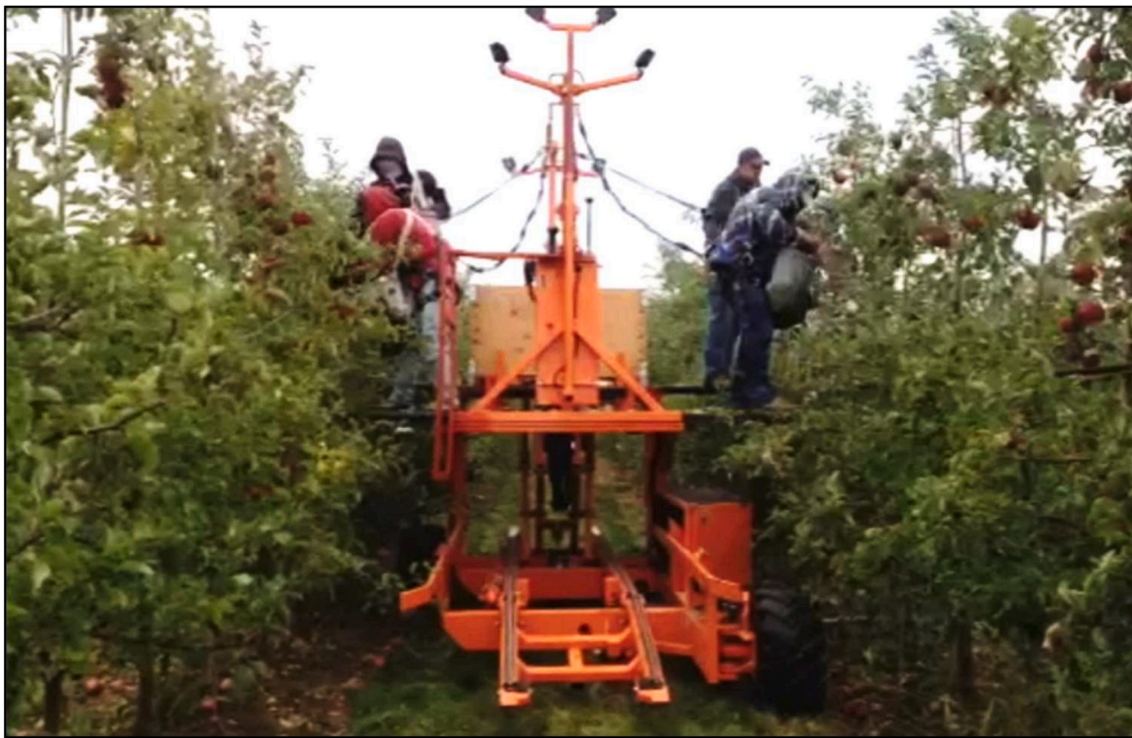
Fig. 1. A harvest-assisted mobile orchard platform.
