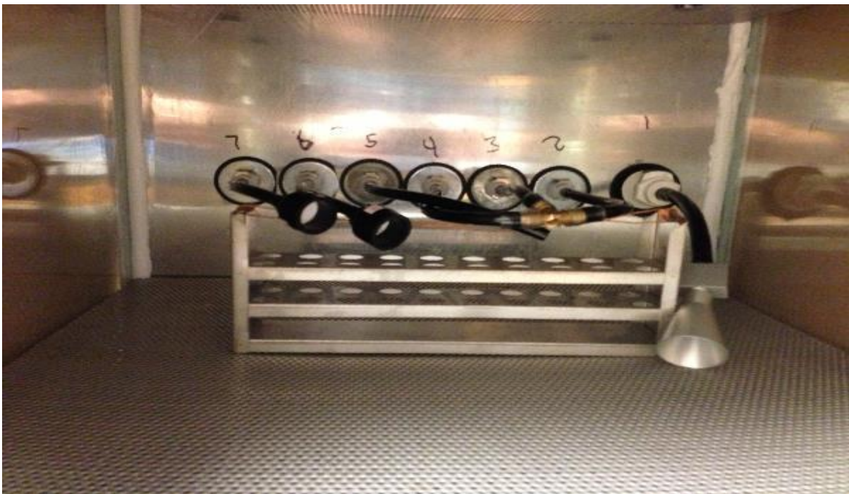
Figure 2: Photograph of sample inlets and sample filters on rack. Note the brass “T” fitting where the SMPS inlets are connected.
