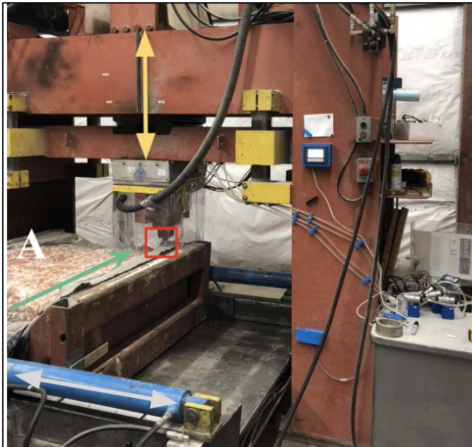
Figure 2. Linear Cutting Machine, where “A” shows the potash rock block cast into the metal box, the red square encompasses the location of the pick within the dust curtain, the green arrow shows the movement of the box under the stationary pick to generate cuts, the white arrows indicate sideways movement of box to index the pick for the next cut, and the yellow arrows show the movement of the frame to control the penetration of cuts.
