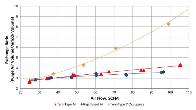
Figure 13. Graph of exchange ratio versus air flow for the tent-type and rigid steel mobile refuge alternative airlocks.
