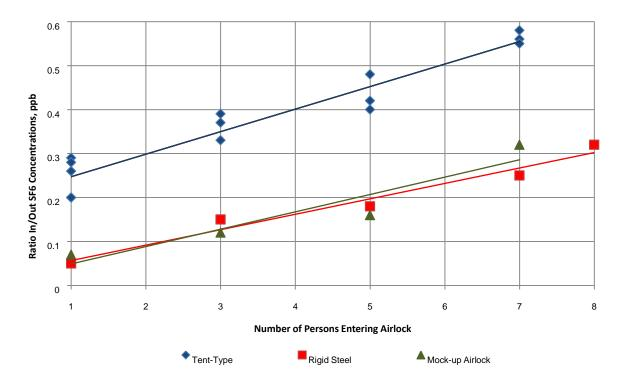
Figure 17. Graph of the ratio of  $SF_6$  concentration (surrogate for carbon monoxide) in the airlock and outside the airlock versus the number of subjects entering the airlock (from data in Table 13).
