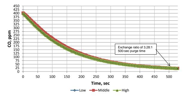
Figure 10. Representative example of data for carbon monoxide (CO) purging of airlock for a rigid steel refuge alternative, test RS-36-0.
