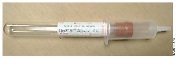
Figure 15. Vacutainer sample tube and needle assembly used to collect SF<sub>6</sub>air samples.
