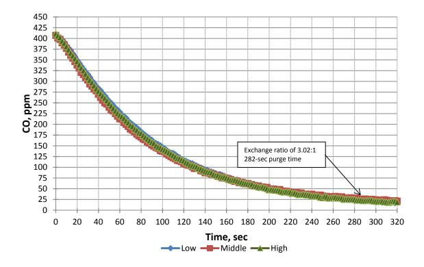
Figure 9. Representative example of data for carbon monoxide (CO) purging of airlock for a tent-type refuge alternative, test TT-25-1.
