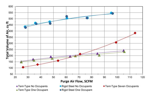
Figure 12. Graph of total volume of air required to purge versus air flow rate.
