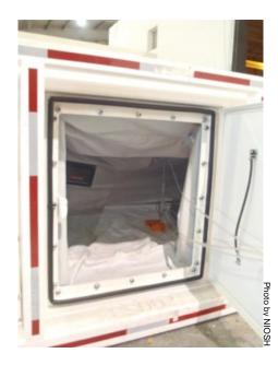
Figure 4. Airlock in a tent-type mobile refuge alternative.
