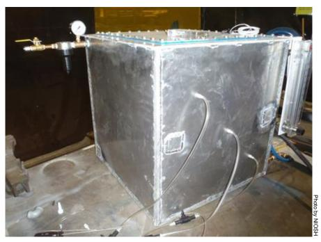
Figure 1. Mini purge box with pressure relief system and sampling ports.
