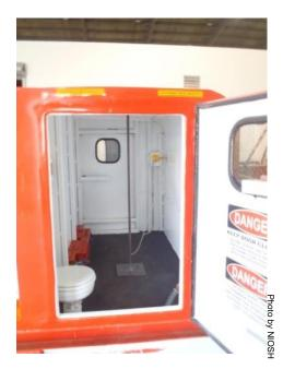
Figure 5. Airlock in a rigid steel mobile refuge alternative.
