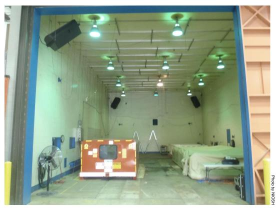
Figure 14. Refuge alternatives in OMSHR's reverberation room in building 154 at the OMSHR Pittsburgh site, Bruceton, PA.
