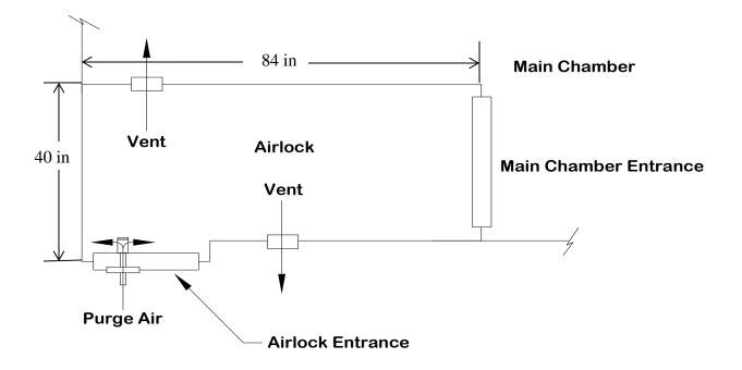
Figure 6. Plan view of air flow schematic for the tent-type refuge alternative airlock during purging.
