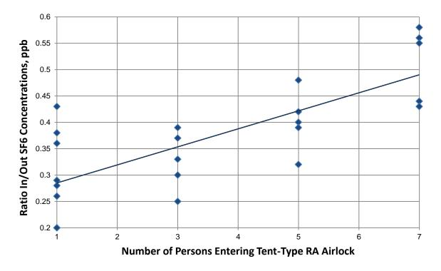
Figure 18. SF<sub>6</sub> contamination ratio versus number of persons entering tent-type refuge alternative airlock at varying entry times.
