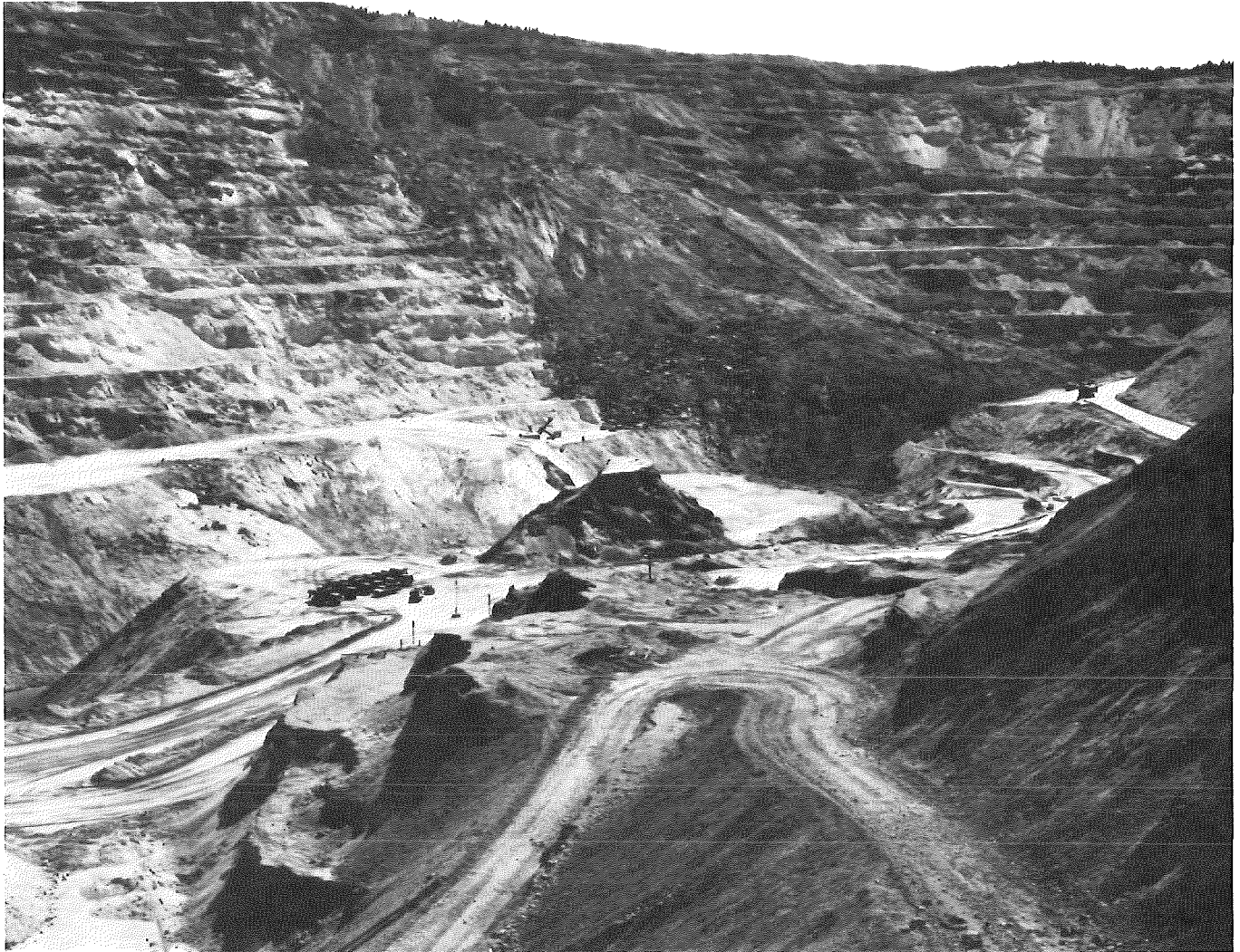
FIGURE 1. - Massive pit wall failure, Liberty Pit, Ruth, Nev.
