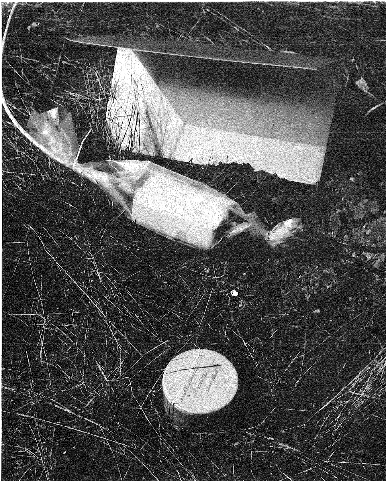
FIGURE 35. - Environmental protection methods for field installation of preamplifier.
