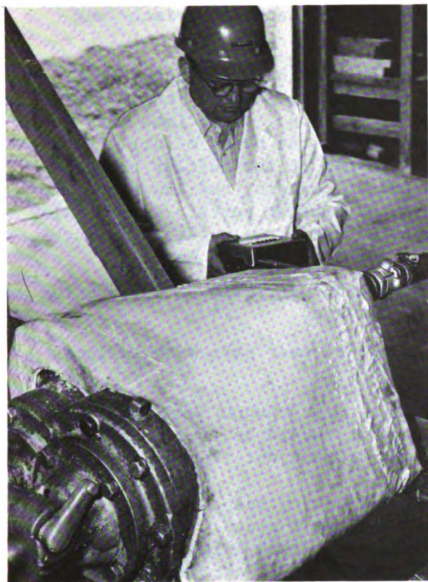
FIGURE 2. - Prototype fiberglass muffler cover installed on the RPD drill.
