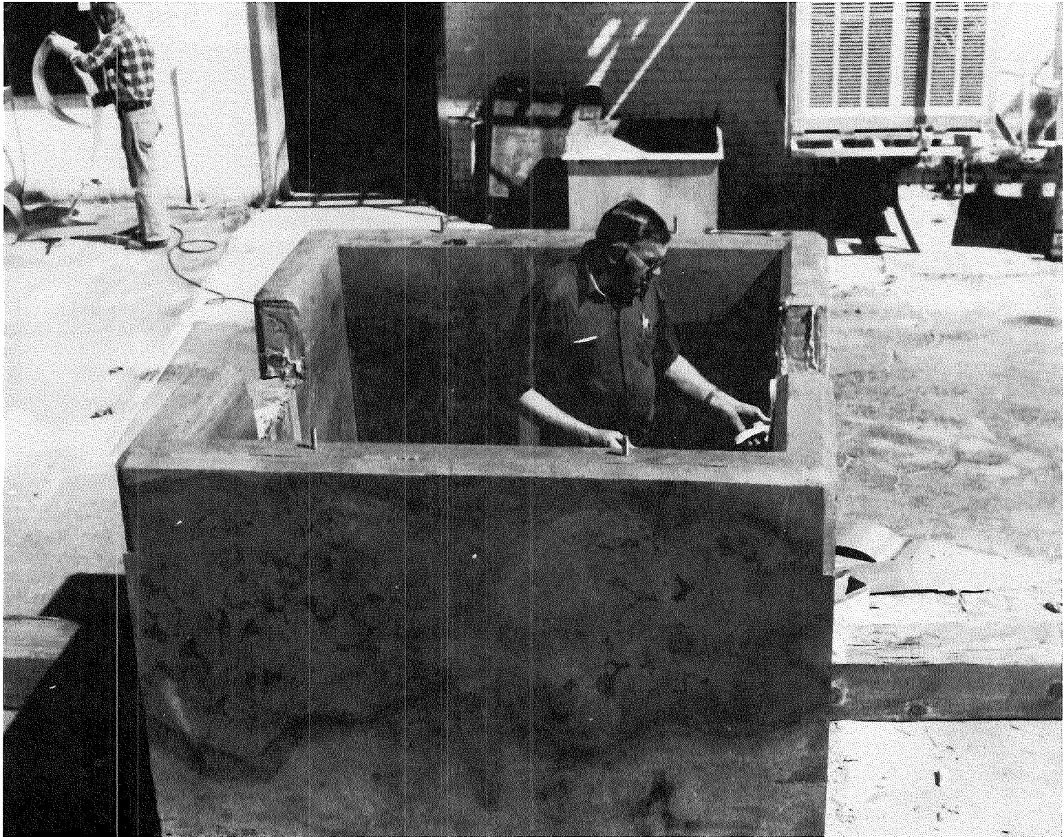
FIGURE 10. - Sulfur concrete sump tank.
