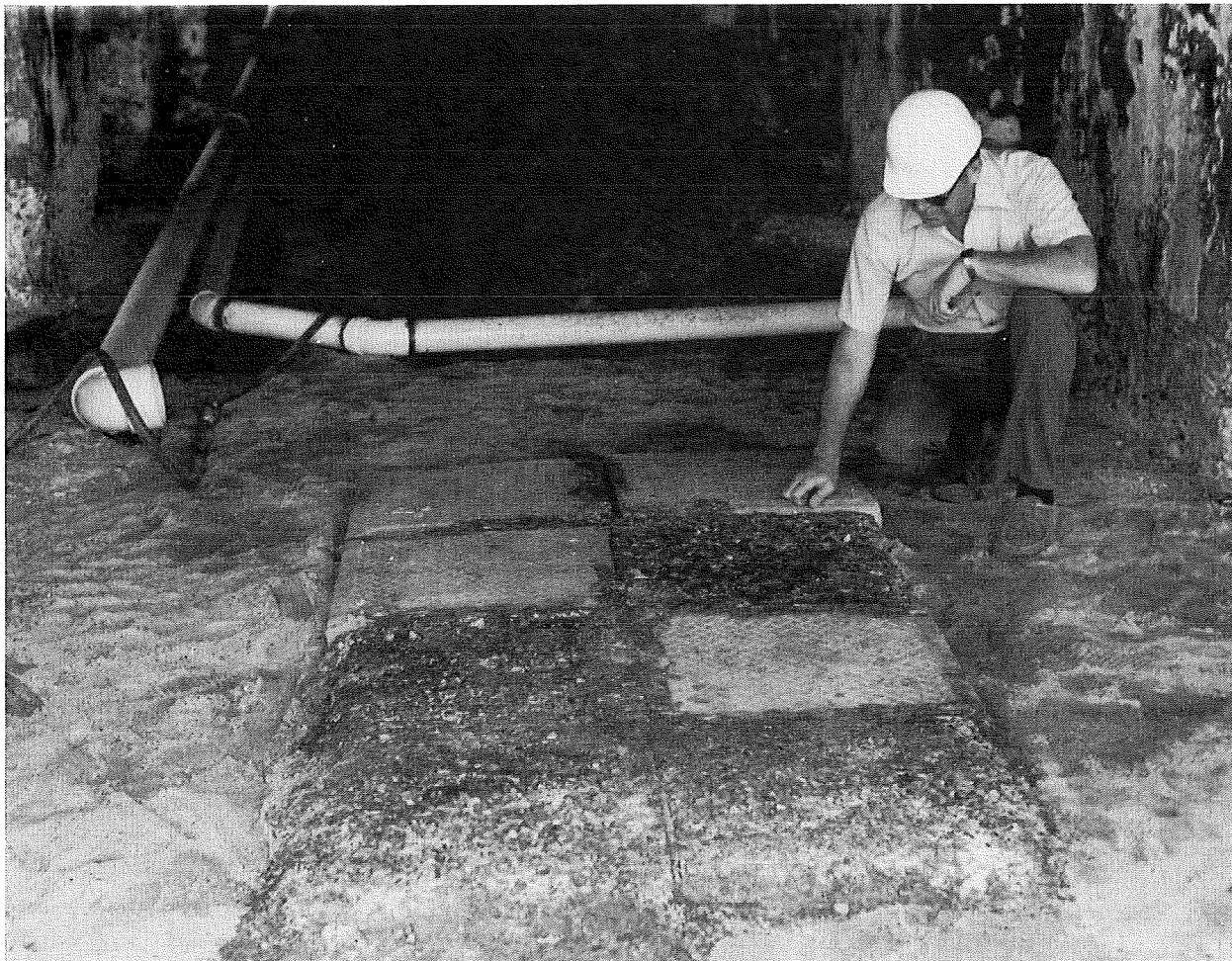
FIGURE 11. - Sulfur concrete test slabs installed with portland cement control slabs in an electrolytic zinc refinery.
