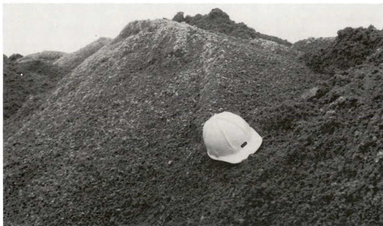
FIGURE 15. - Agglomerated feed for the 1,000-ton pilot-scale heap leaching experiment near Lovelock, Nev.
