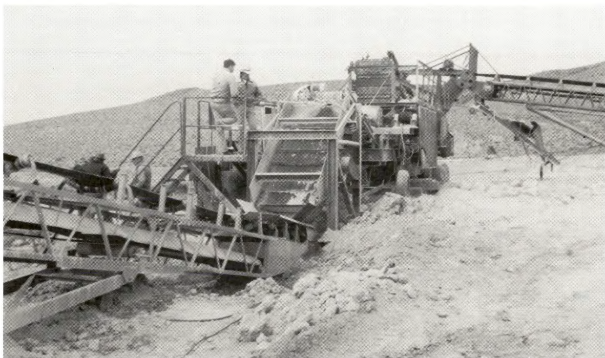
FIGURE 14. - View of agglomerator used in pilot-scale agglomeration experiment conducted near Lovelock, Nev.
