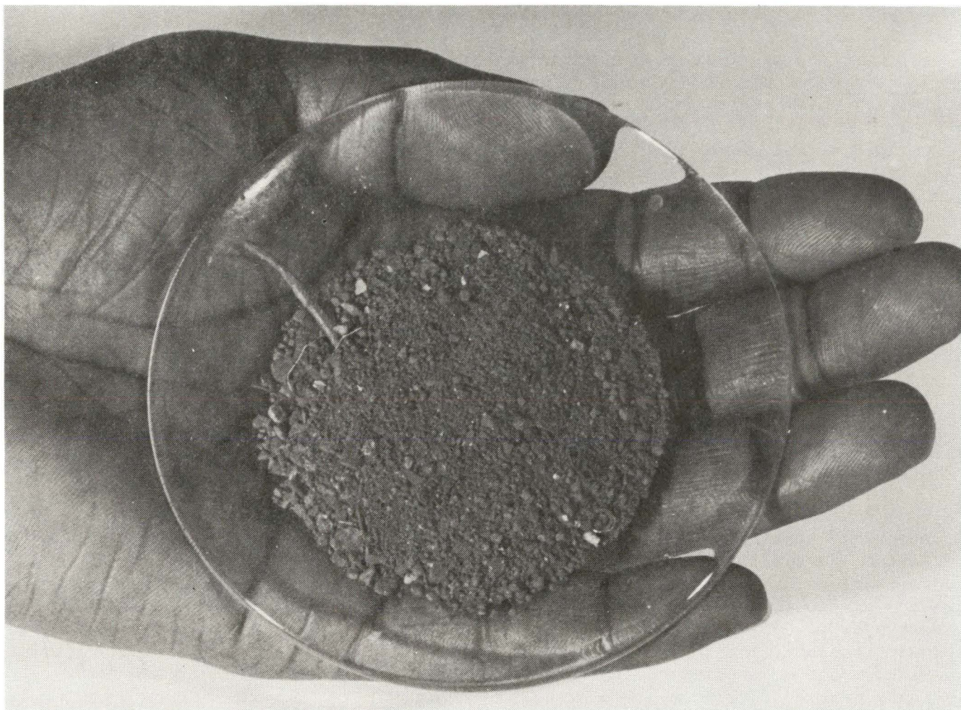
FIGURE 5. - Final residue produced after third-stage leach and wash.
