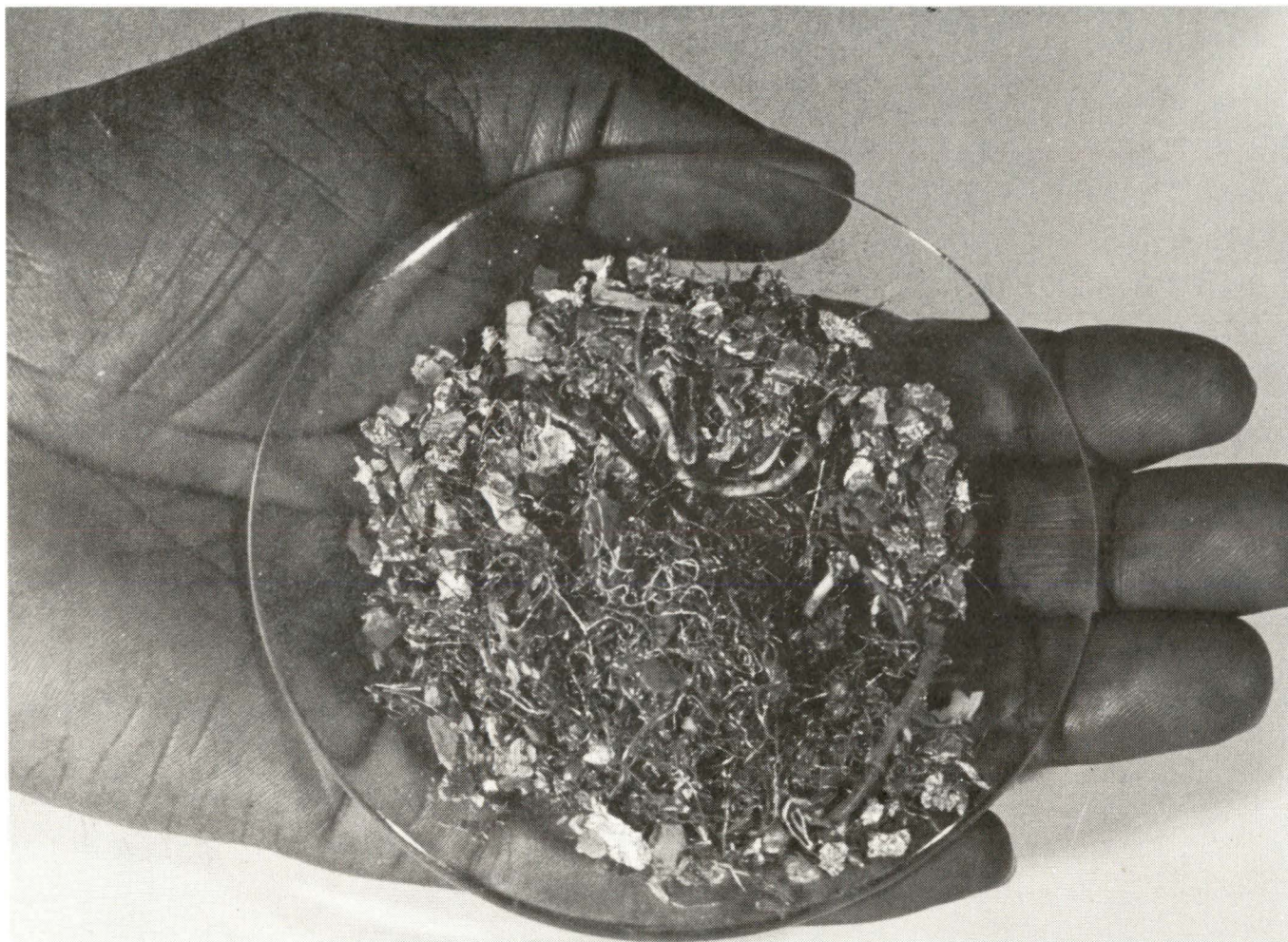
FIGURE 3. - Typical HTS fractions (minus 1/4-in nonmagnetic metallic concentrates) from processed electronic scrap.
