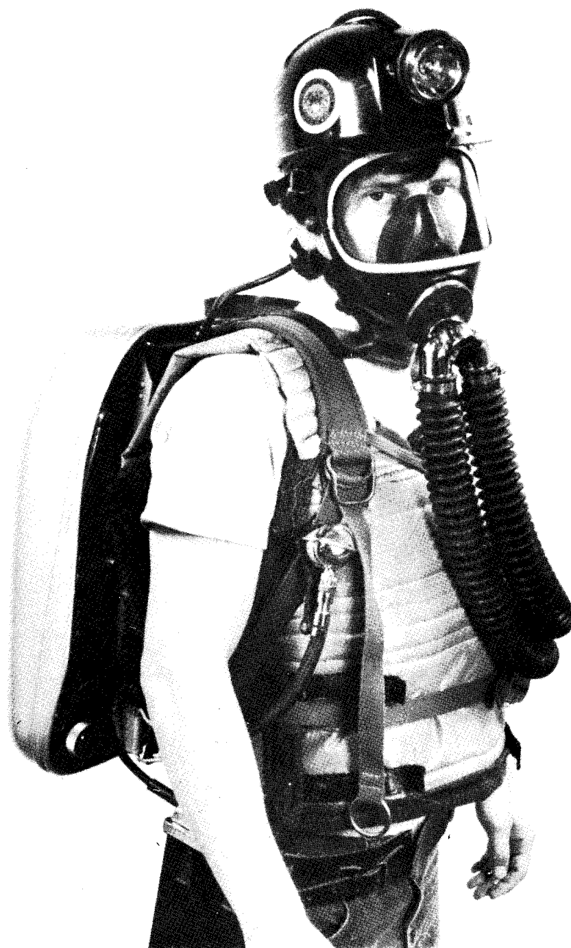
FIGURE 3. - Bureau of Mines ice-cooling garment worn with a breathing apparatus.
