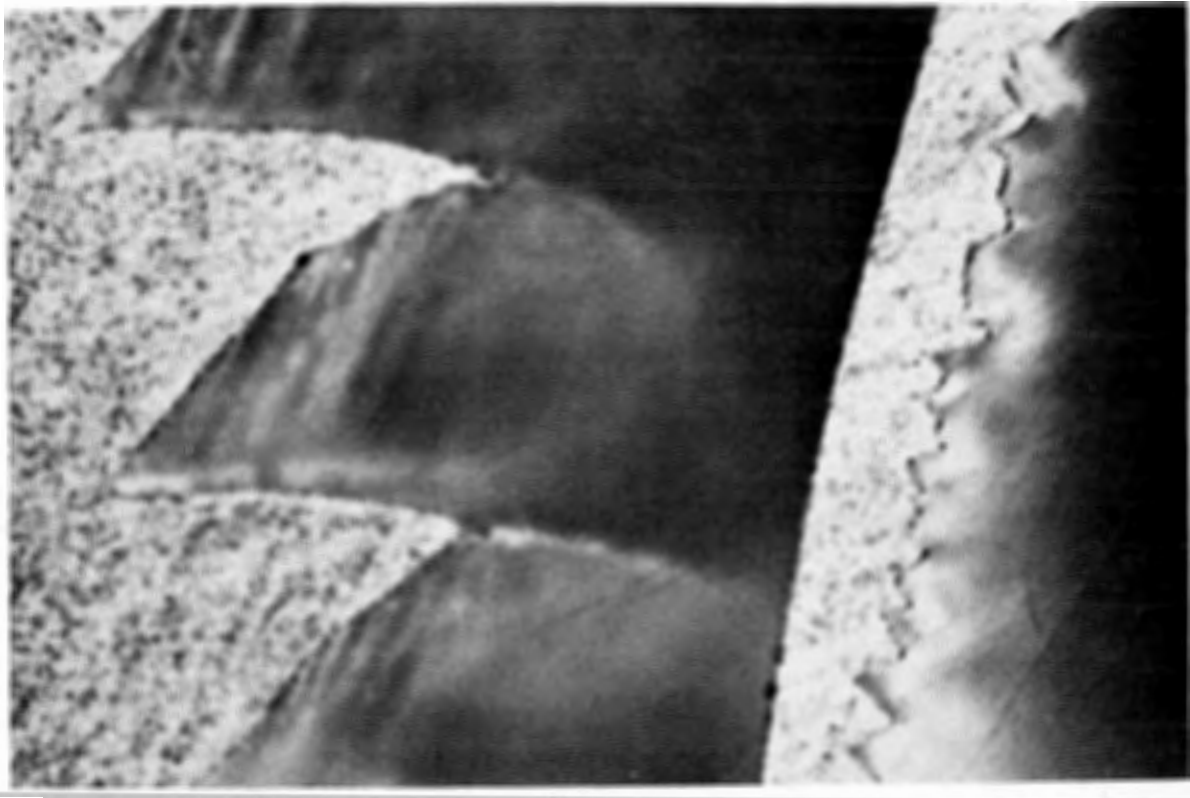
FIGURE 2. - Cross Section of Titanium Alloy Shaving Segments.
