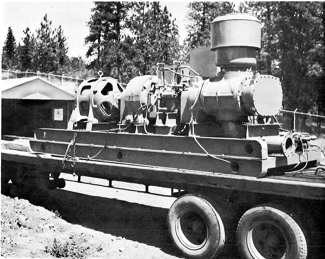
FIGURE 10. - Three-hundred-hp motor, eddy current coupler, and speed increaser to blower.
