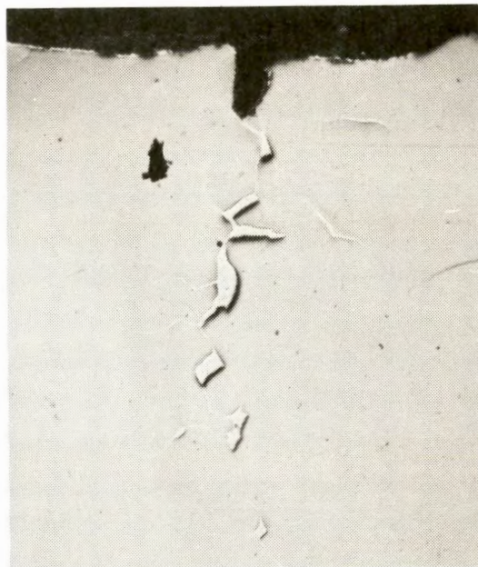
FIGURE 2. - Penetration of Copper Into Steel Rolled at 2,370° F (1,300° C), X 50.
