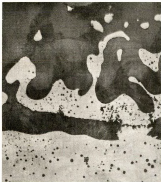
FIGURE 14. - Absence of Copper on Surface of Steel Containing Boron and Silicon After Scaling at 2,100° F (1,150° C), X 500.
