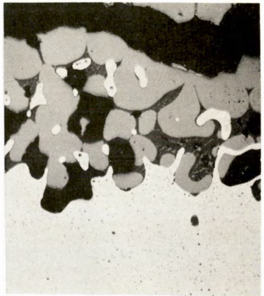
FIGURE 12. - Absence of Copper on Surface of Steel With 0.16 Pct Si When Scaled at 2,200°F (1,205°C), X 500.
