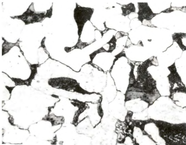
FIGURE 8. - Structure of steel 146 containing 0.2 wt-pct C, 0.8 wt-pct Cu, and 0.19 wt-pct Si. (X 1,000)
