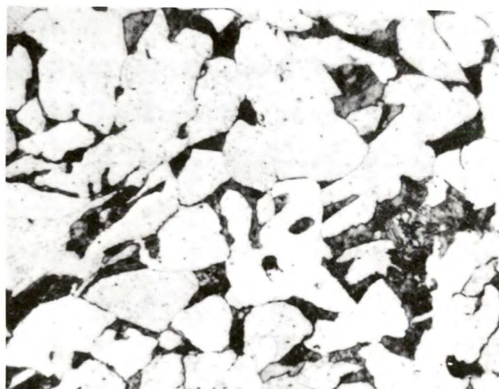
FIGURE 9. - Finer structure of steel 149 containing 0.2 wt-pct C and 0.8 wt-pct Cu, but with 1.13 wt-pct Si. (X 1,000)
