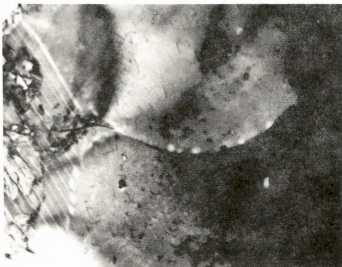
FIGURE 10. - Absence of copper in hot-rolled steel 118 containing 1.05 wt-pct Cu. (X 50,000)
