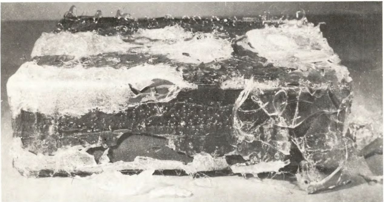
FIGURE 9. - Cellulose Acetate Butyrate Plastic Coating on Rock Slab.
