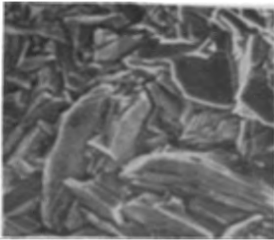
FIGURE 4. - 6-hour deposit, 1 mg/l Ti in the electrolyte (X 1,000).
