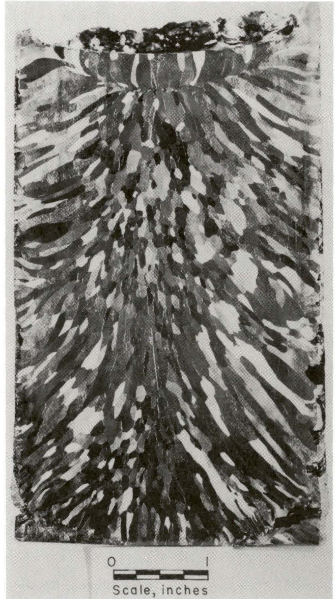
FIGURE 11. - As-cast macrostructure of TZM ingot prepared by consumable-electrode-arc melting in a cold copper crucible.
