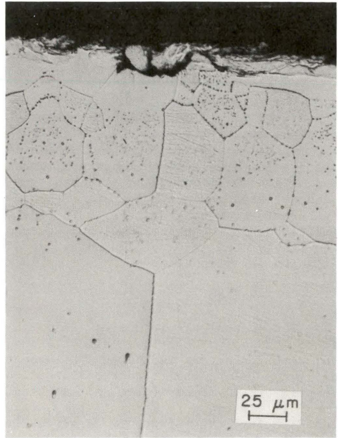
FIGURE 13. - Optical micrograph showing TZM structure in figure 12 at greater magnification (X 400).
