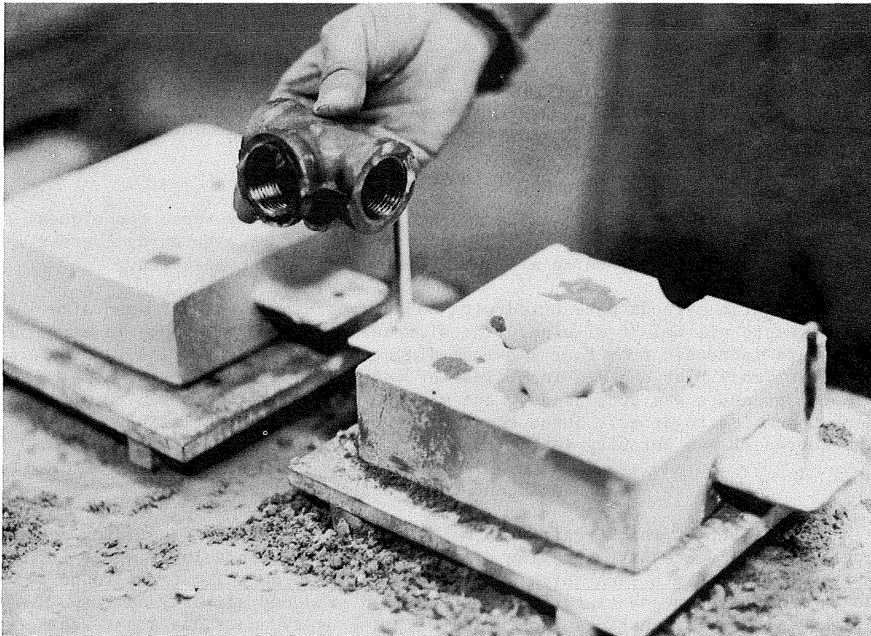
FIGURE 5. - One-inch titanium pipe tee and zirconia-washed olivine mold with core in place.
