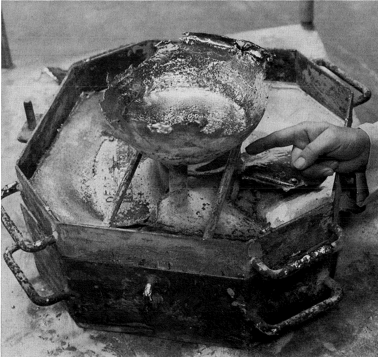
FIGURE 12. - Cope view of titanium propeller cast in zircon mold bonded by western bentonite and dried at 980° F (525° C).
