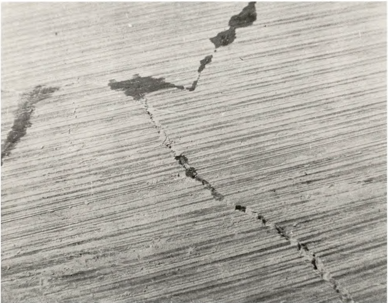
FIGURE 3. - Penetration of monomer into shale rock.
