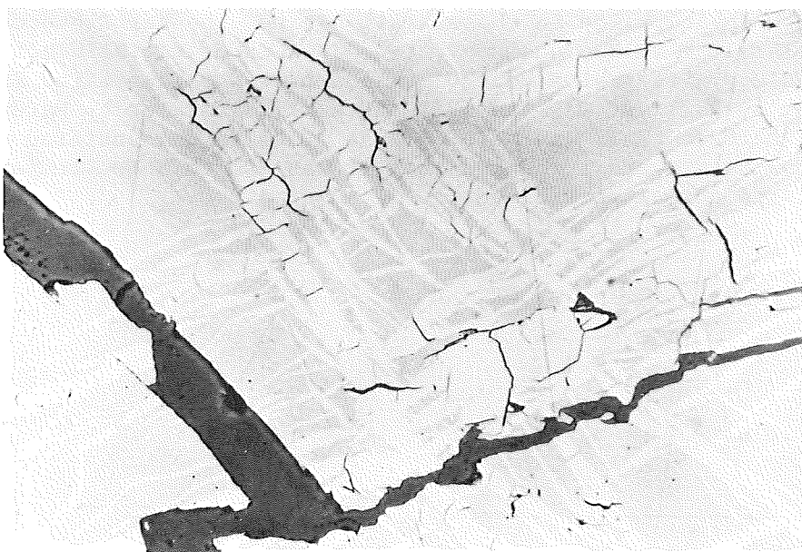
FIGURE 26. - Almost complete replacement of pentlandite by chalcopyrite-cubanite. 2,520.0 feet; reflected light (X 400). Only what appear to be pentlandite veinlets (light gray) are left. Chalcopyrite-cubanite intergrowths (gray) have replaced the pentlandite from the cleavages into the grain from both sides leaving a two-directional network of pentlandite. Eventually, these resemble flames and could be construed as a primary texture. The dark-gray phase is silicate.
