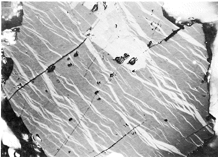
FIGURE 20. - Pyrrhotite-troilite intergrowth, 2,554.2 feet; reflected light, oil immersion (X 150). Pyrrhotite (dark gray), troilite (light gray wavy stripes) with chalcopyrite-cubanite intergrowth (top center, two shades of gray, blocky stripes). Silicate matrix on left and right sides.
