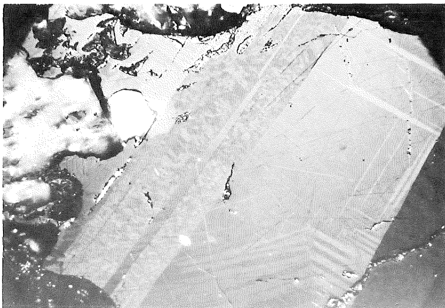
FIGURE 28. - Cubanite lamellae showing patchy extinction. 2,523.9 feet; reflected light, partly crossed polars (X 80). Cubanite in central area (mottled stripes elongated northeast-southwest) cutting chalcopyrite (twinned). These patchy areas are probably due to inversion of the cubanite to a lower temperature form.
