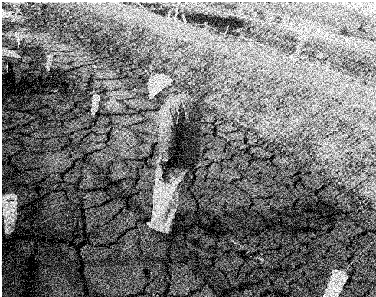
FIGURE 9. - Partially dewatered fine coal-refuse slurry.
