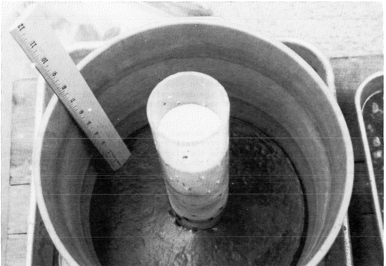
FIGURE 1. - Laboratory slurry-dewatering test equipment.
