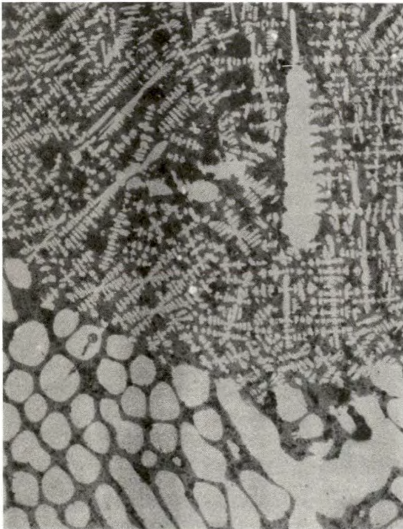
FIGURE 2. - Microstructure of specimen quenched from the liquid plus Y 2 O 3 solid solution region: SrF 2 -60 mole-pct Y 2 O 3 , heat-treated ¼ hour at 2,200°C, held ½ hour at 2,000°C, quenched in oil. Magnification X 125.
