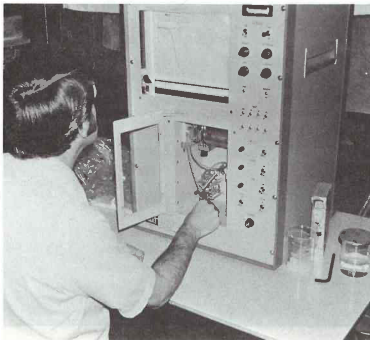
FIGURE 7. - Sedigraph 5000 for determining minus 200-mesh particle size.
