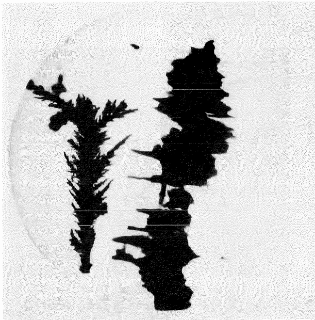
FIGURE 9. - Dendritic Growths Resulting From Unfavorable Conditions (X 150).
