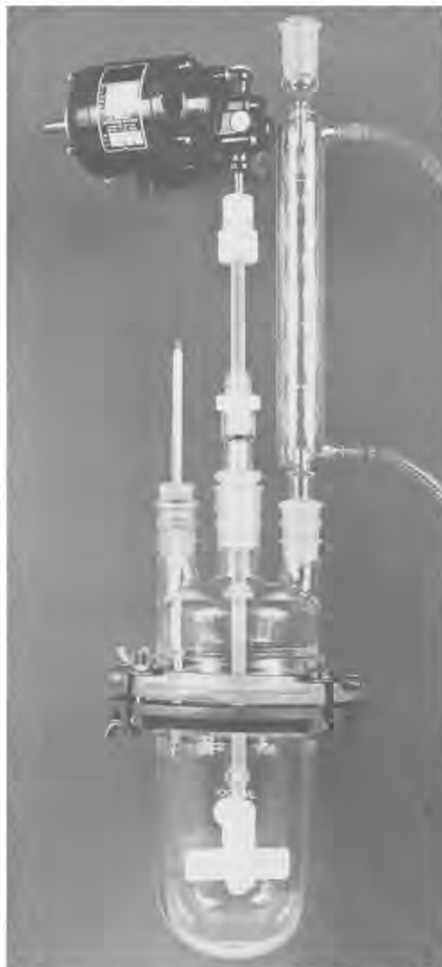
Figure 4.—Bench-scale reactor for producing 500-mL resin batches.
