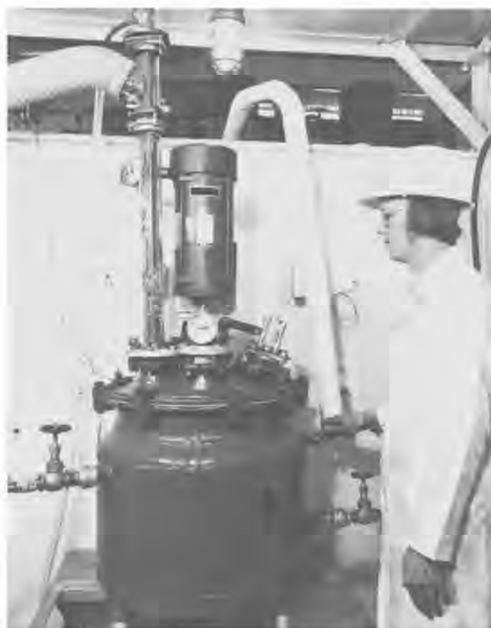
Figure 6.—Semicommercial reactor for producing 1-ft 3 resin batches.
