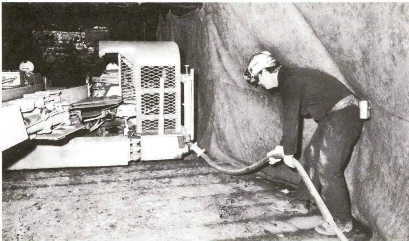
Figure 1.—Miner handling trailing cable underground.
