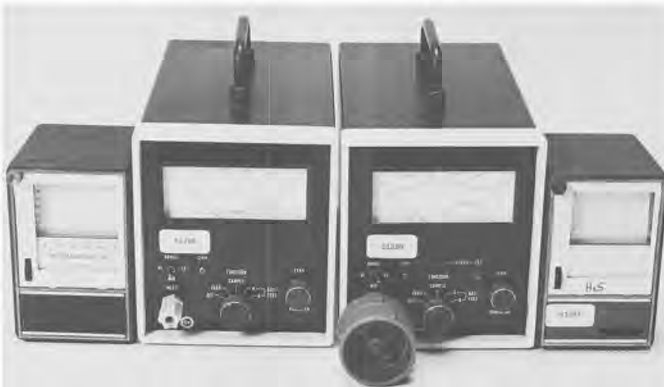
Figure 25.—Recording instruments for measuring hydrogen sulfide and sulfur dioxide concentrations.
