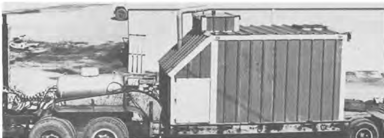
Figure 23.—SC transporter with heating and mixing system (10-yd 3 capacity).
