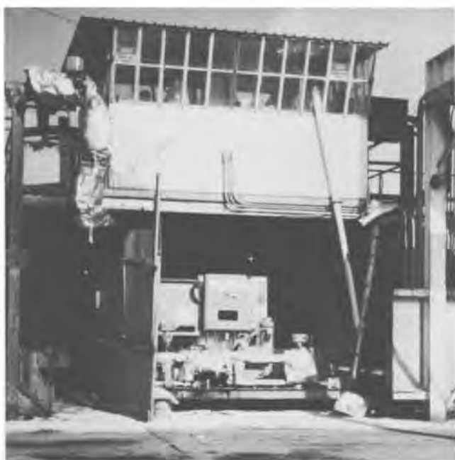
Figure 45.—Modified asphalt mix plant for preparing SEA pavement using colloid mill to disperse sulfur in asphalt.
