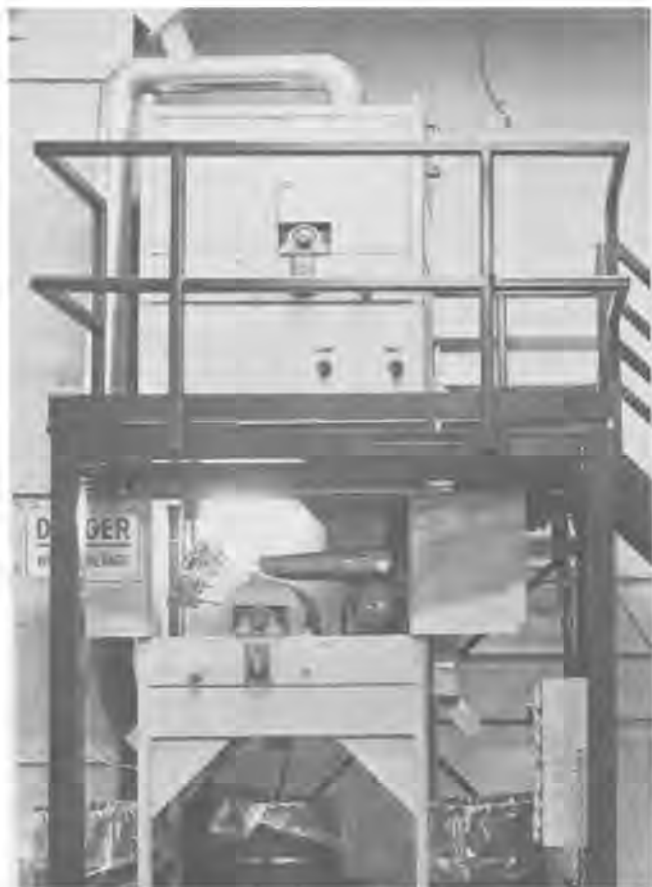
Figure 18.—Two-stage, high-tension separator used to recover aluminum.
