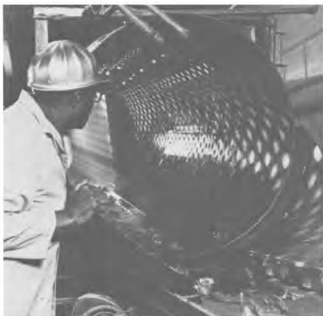
Figure 5.—Trommel used for wet-screening incinerator residue.
