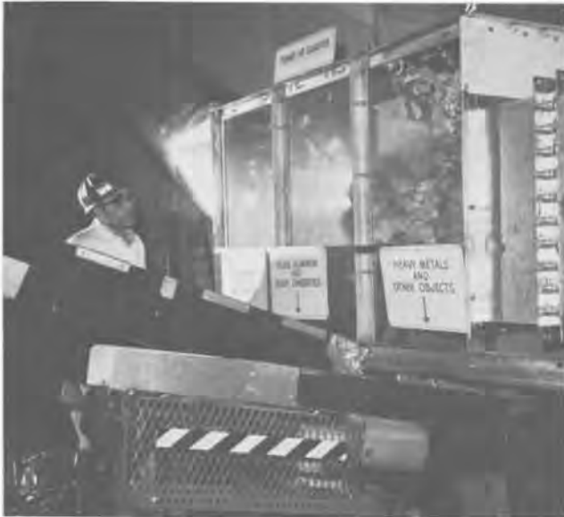
Figure 13.—Horizontal air classifier making a three-way separation.
