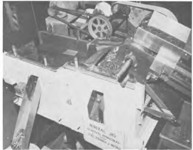
Figure 15.—Mineral jig used to recover a coarse glass concentrate.
