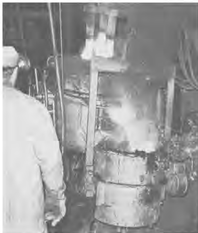
Figure 20.—Test ladle (1½ st) receiving molten iron from arc furnace.
