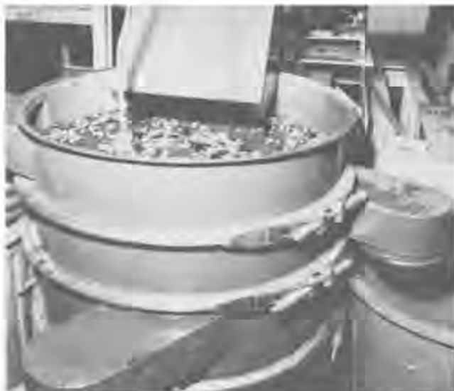
Figure 6.—Screening and washing nonferrous metals.
