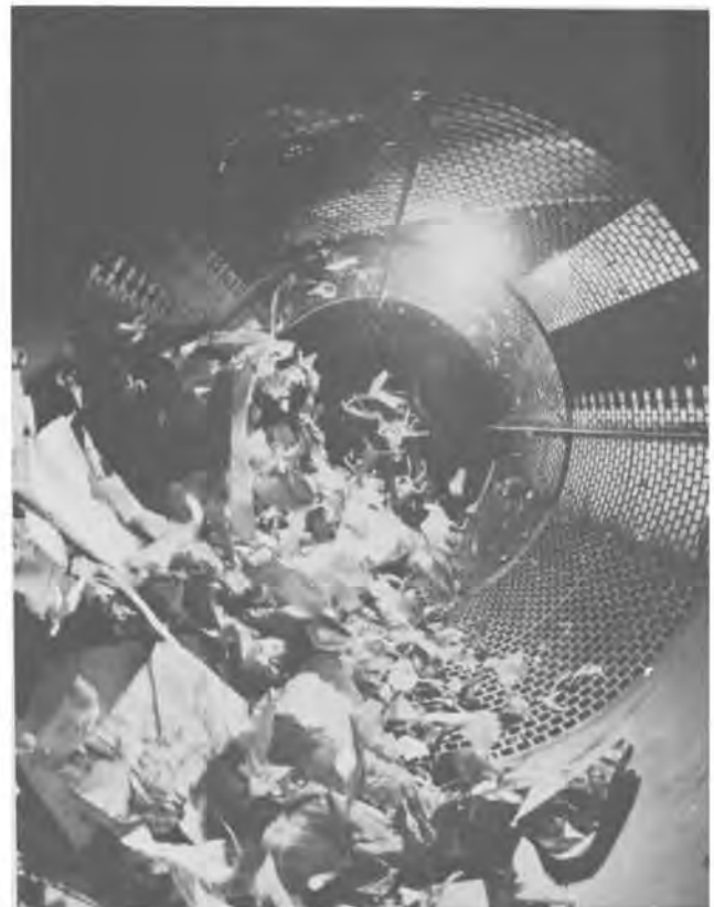
Figure 16.—Three-stage aspirator separating paper and light plastic from aluminum and heavy combustibles.
