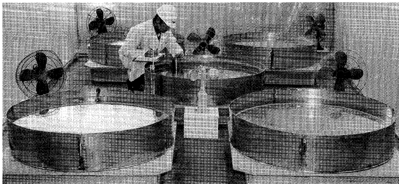
FIGURE 1. - Evaporation pans and monitoring equipment for potash brine evaporation studies.
