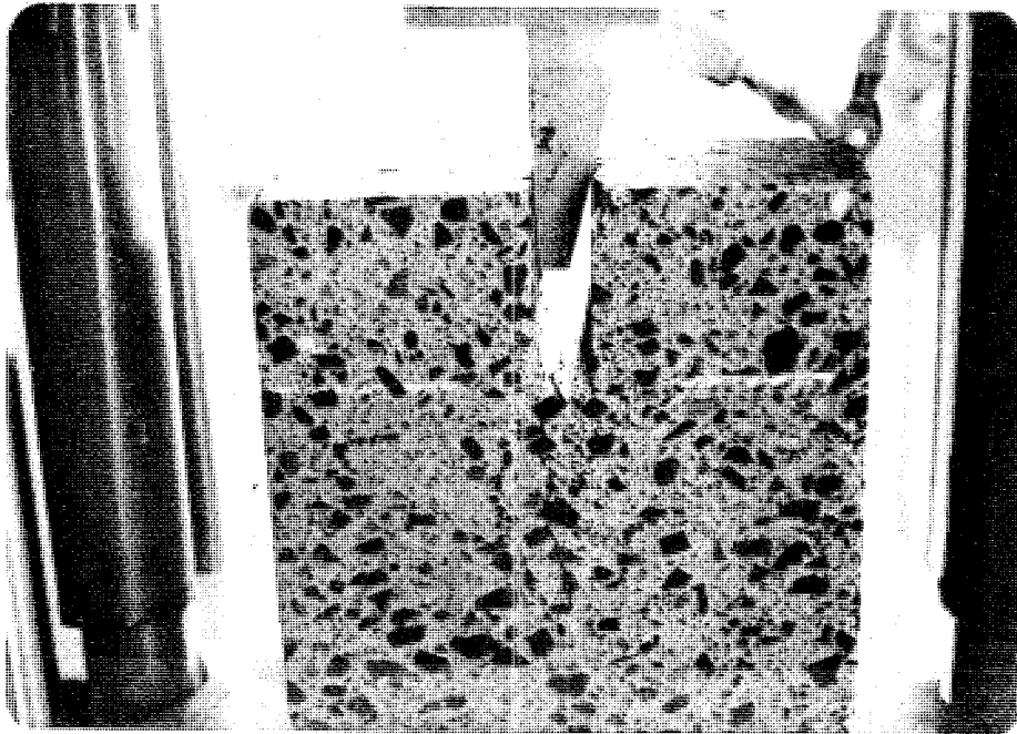
Figure 6.4. Configuration of wedge test to determine "ploughability" of the artificial coal from Bruceton.
