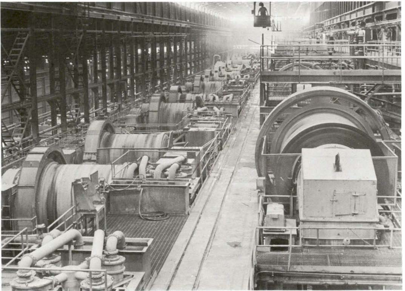
FIGURE 1.—Grinding section of a copper ore processing operation.
