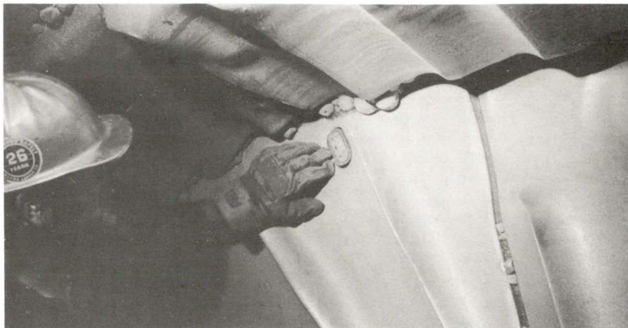
FIGURE 11.—Installed electrode assembly.
