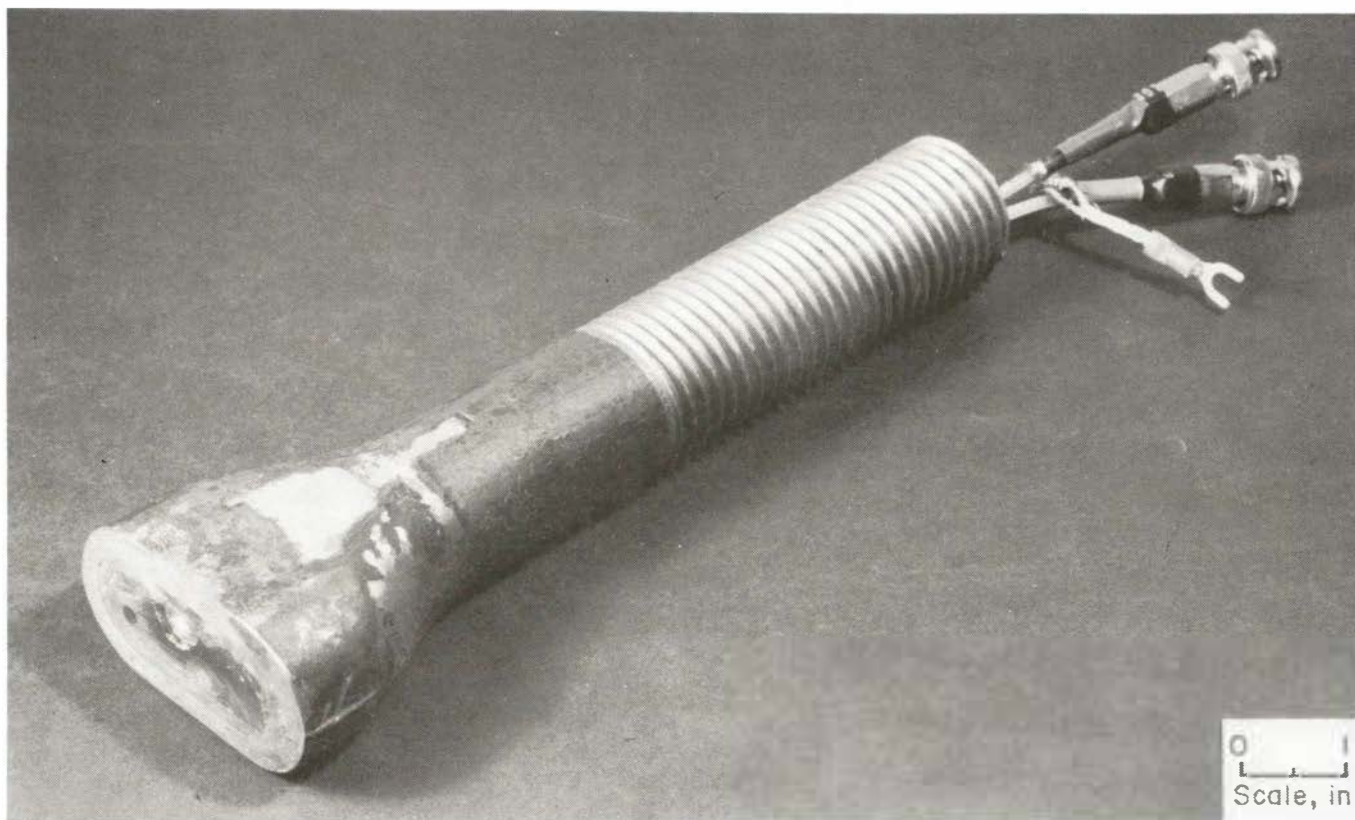
FIGURE 8.—Electrodes mounted in mill liner bolt for field tests. (See also figure 9.)
