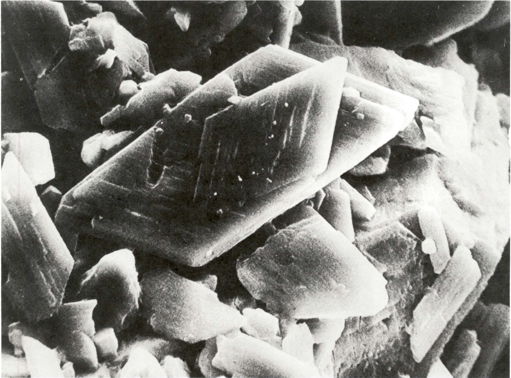
FIGURE 2. - Scanning electron microphotograph of phosphogypsum (X 1,000).
