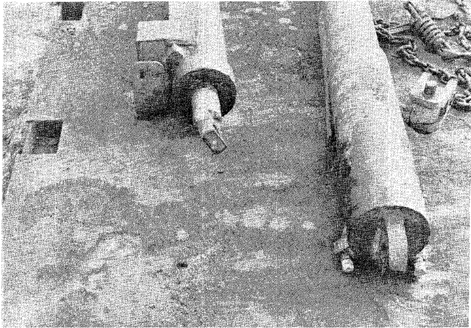
RIGHT RAM CYLINDER ROD END BENT
