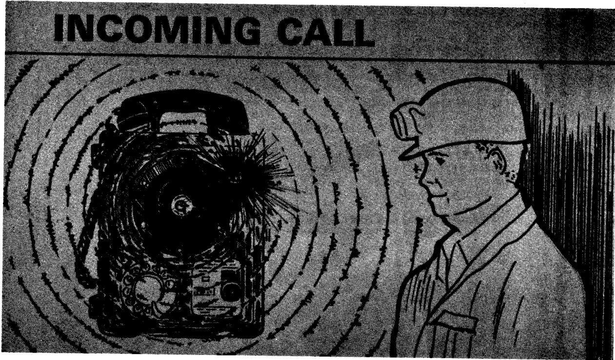
FIGURE 5. - System notifies called party by "birdie" tone signal (optional flashing light also indicated).
