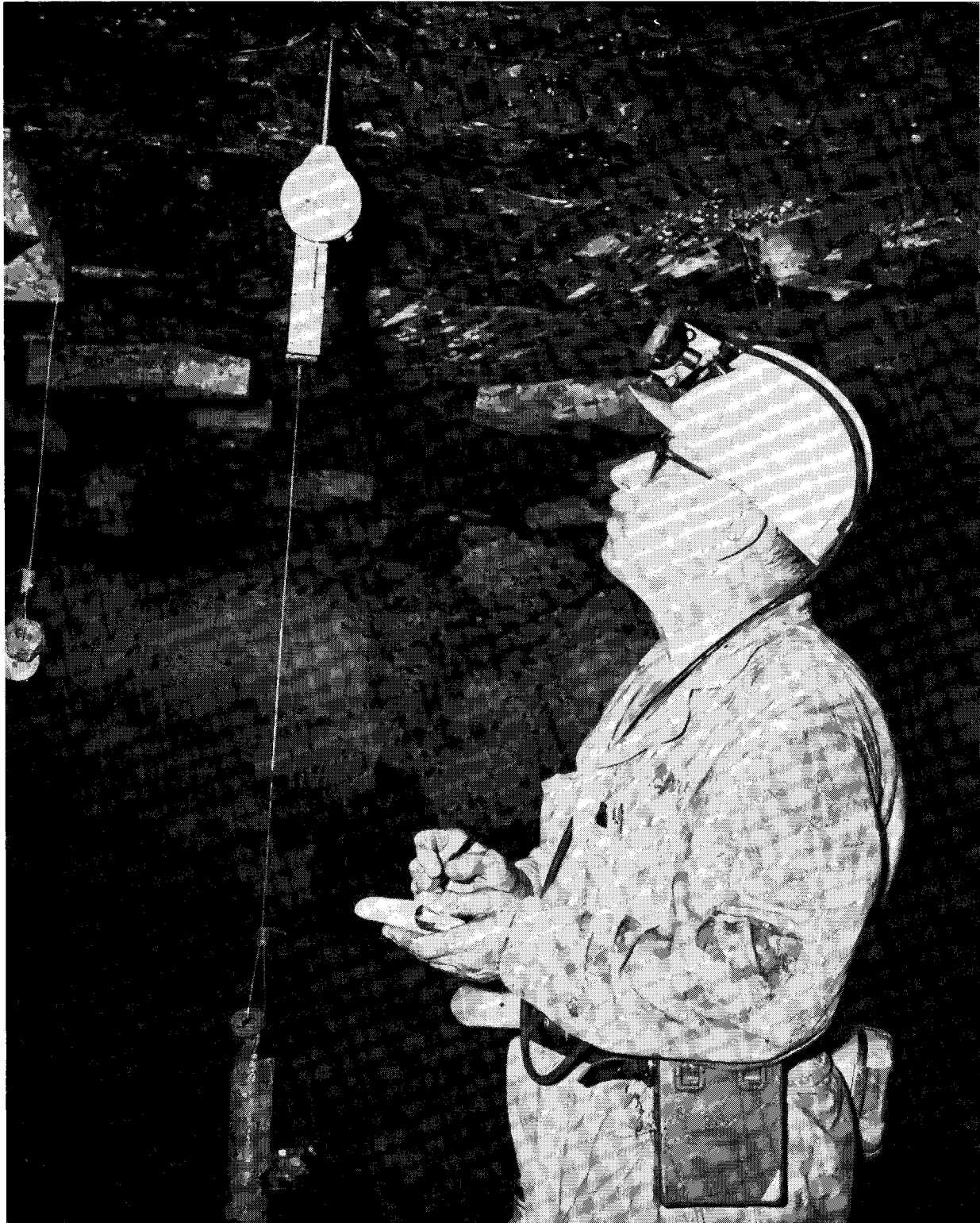
FIGURE 13. - Using 10-Horizon Spring-Anchor Piano-Wire Extensometer To Measure Roof Strata Separations in 70-Foot Borehole Near Longwall Face.
