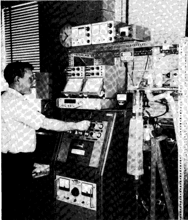
FIGURE 12. - Developing Analyzer for Size and Concentration of Dust in Stack Gases.
