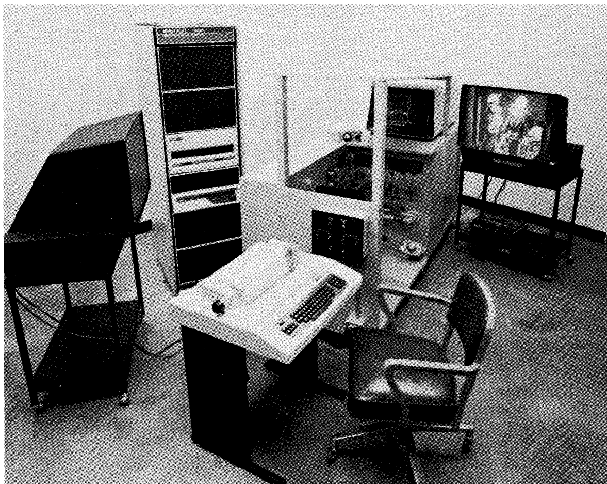
FIGURE 5. - Continuous miner part-task trainer.
