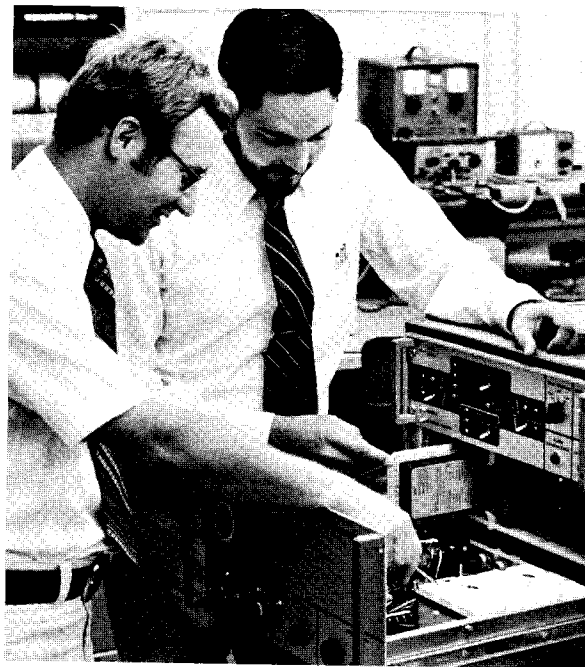
FIGURE 7. - Mine shaft fire and smoke protection system, surface control unit.
