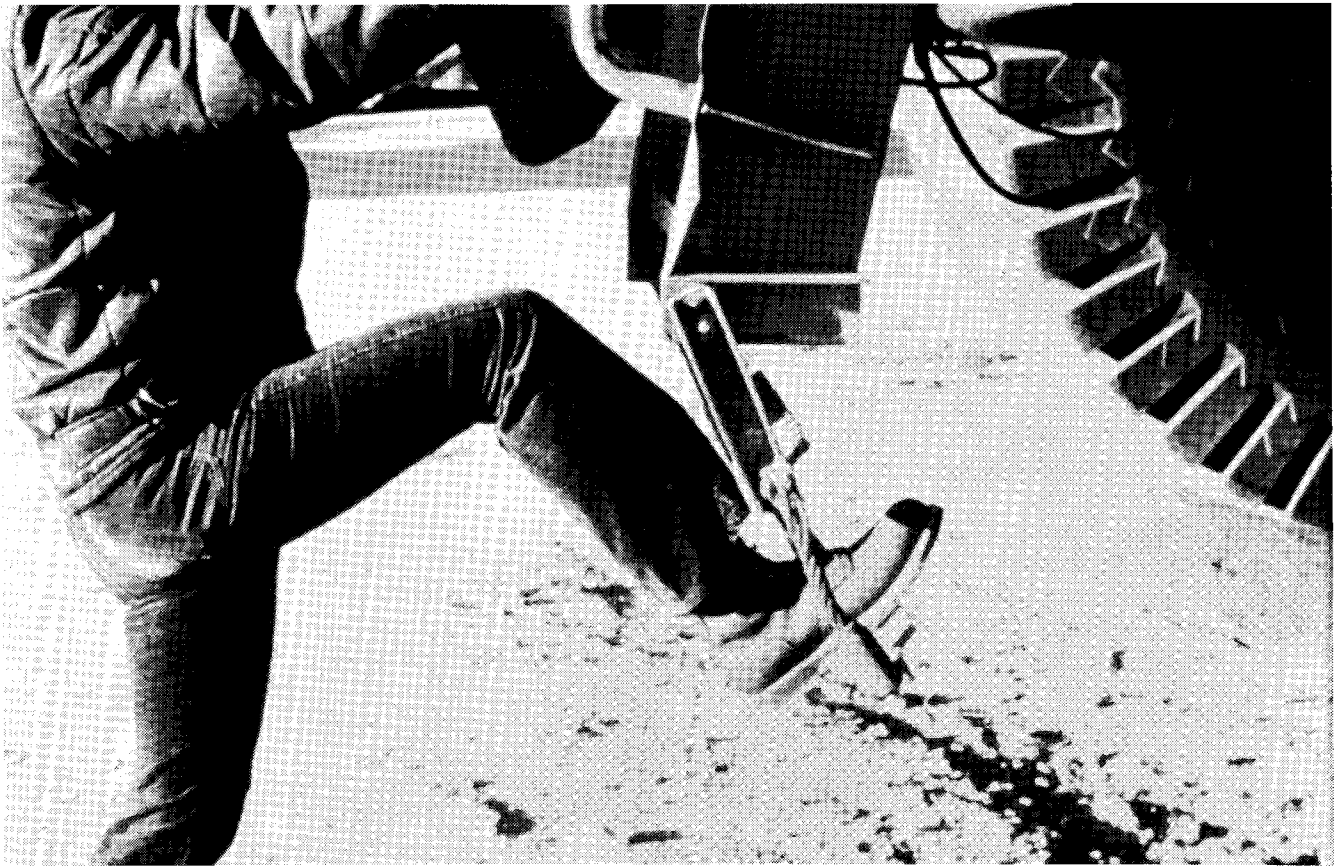
FIGURE 6. - Cable ladder showing lack of rigidity when stepped on.
