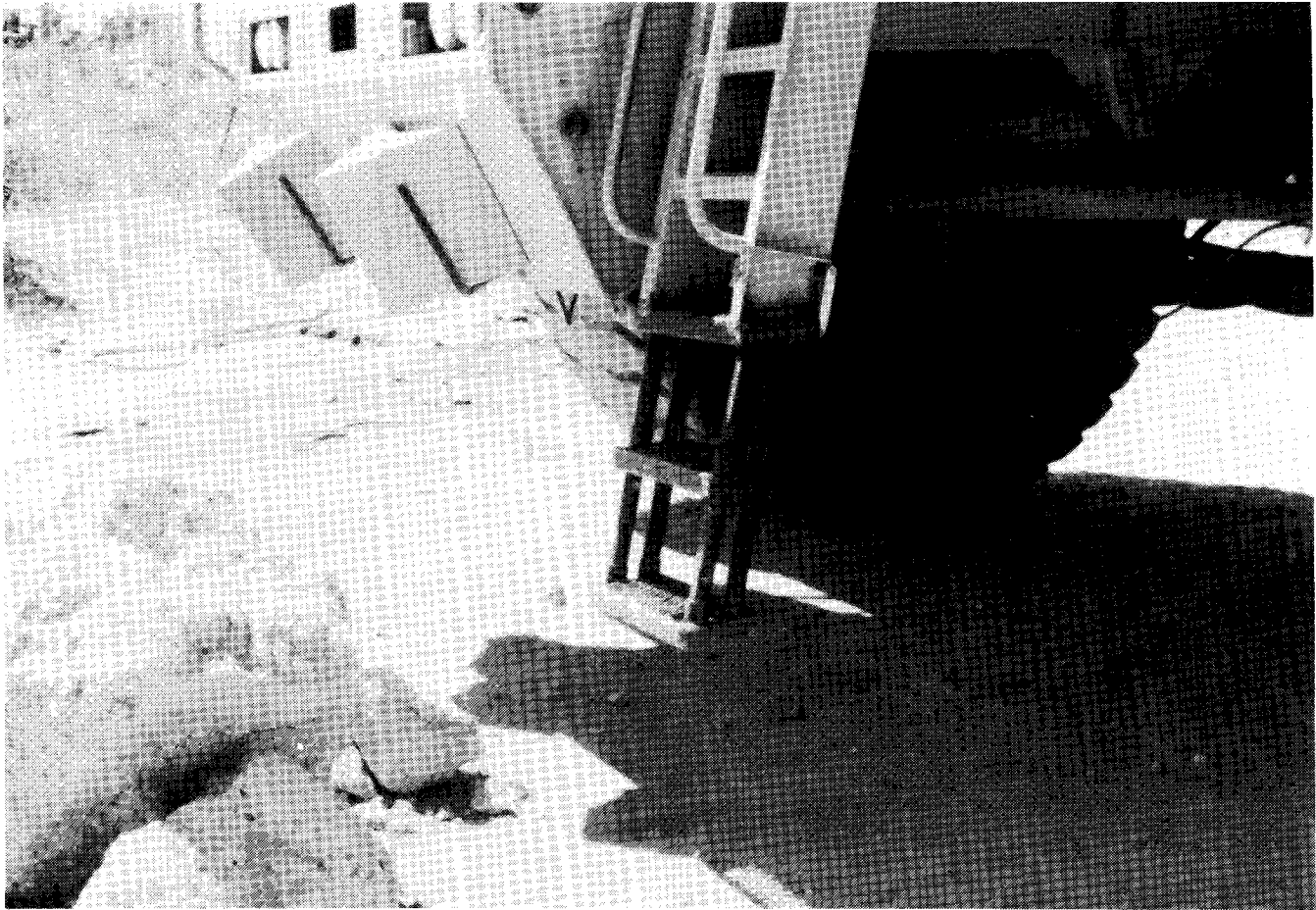
FIGURE 8. - Spring step retrofitted to truck ladder.
