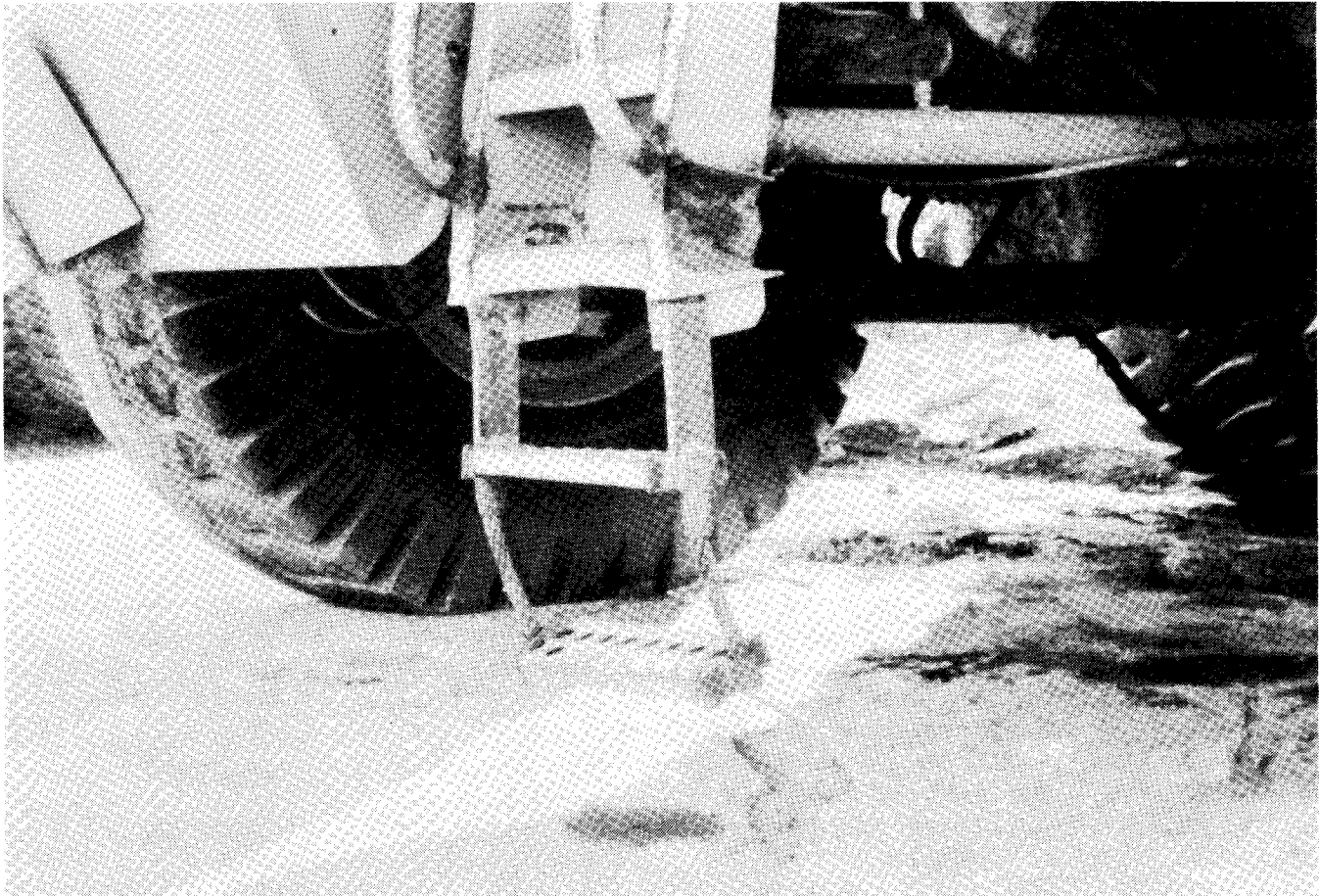
FIGURE 1. - Typical ladder on off-highway haulage truck.
