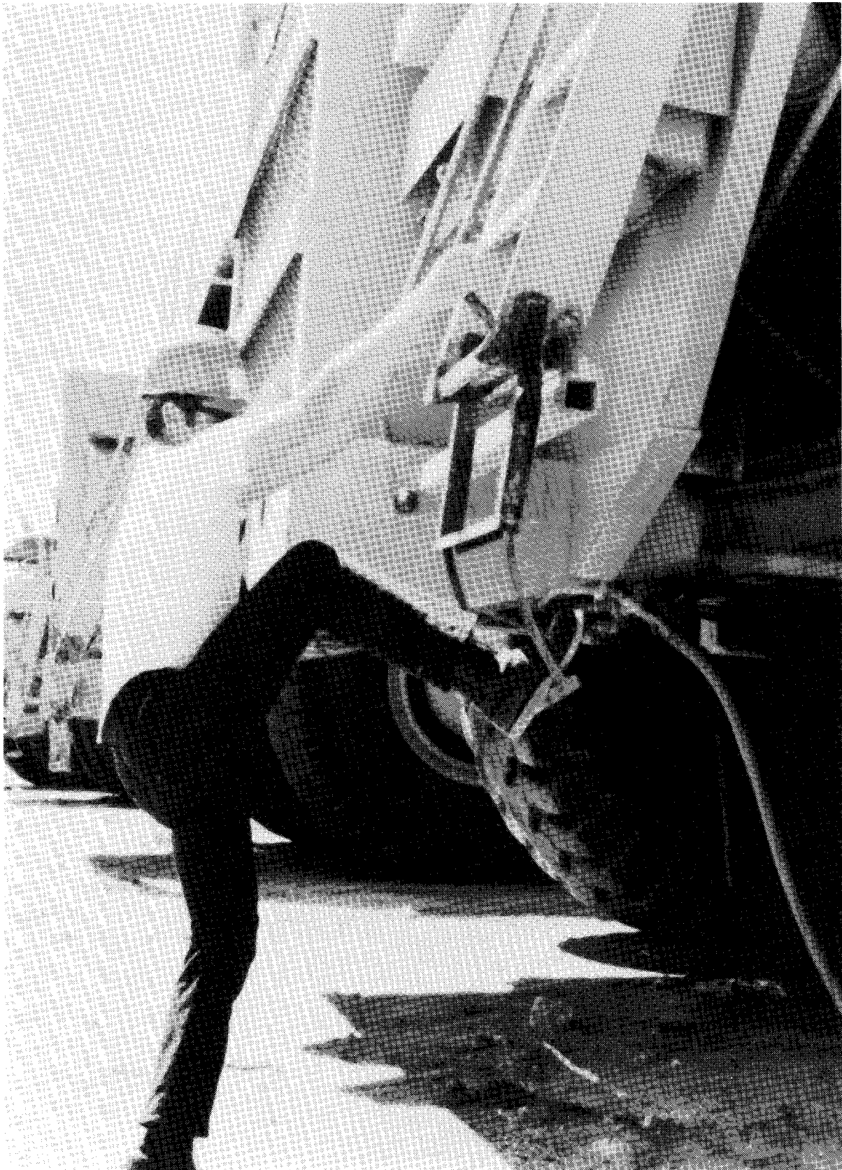
FIGURE 5. - Cable ladder showing height of first step.
